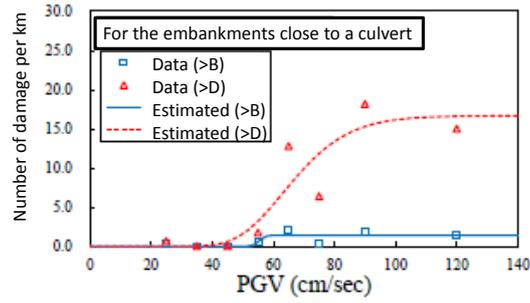
(a) For the embankments close to a culvert
