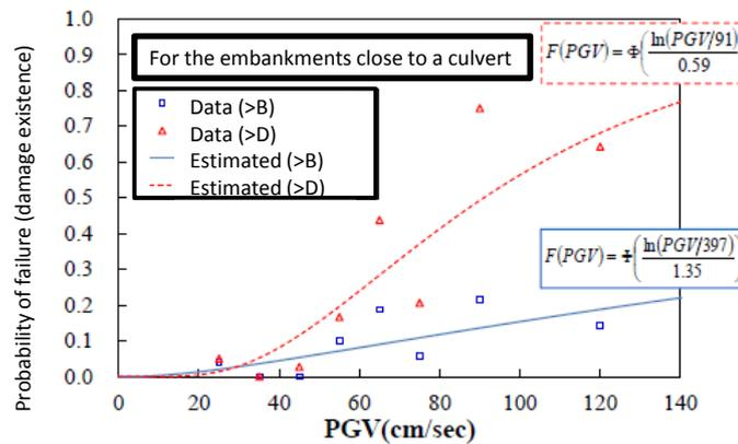
(a) For the embankments close to a culvert
