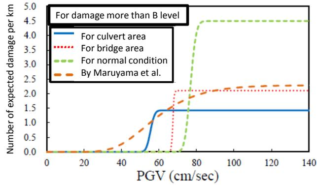
(a) Fragility curves for the damage more than B level
