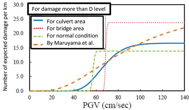
(b) Fragility curves for the damage more than D level
