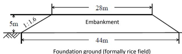
**Figure 1.** The typical cross section of embankment considered in this study
