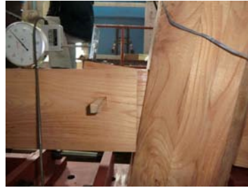
Fig.23 Partial compressive deformation.
