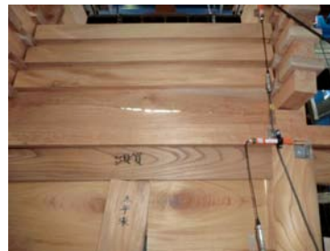
Fig.25 Crack of board wall.
