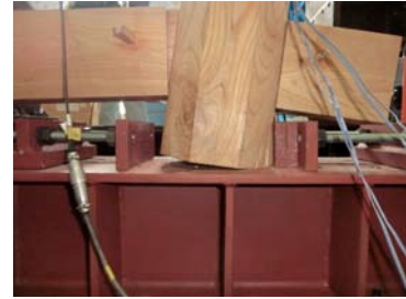
Fig.24 Rotation of the bottom of the column.
