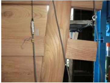
Fig.23 Partial compressive deformation.
