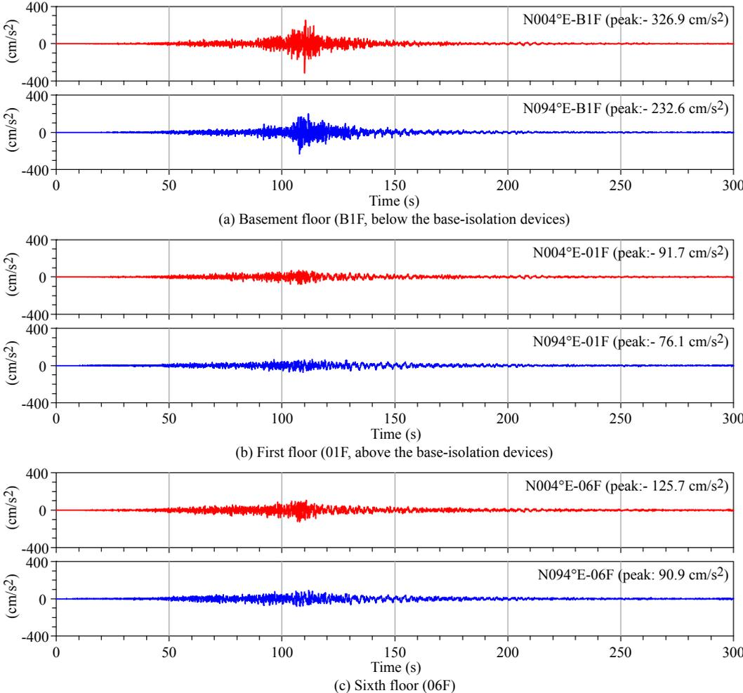
Figure 6. Acceleration waveforms recorded in the TKC building
