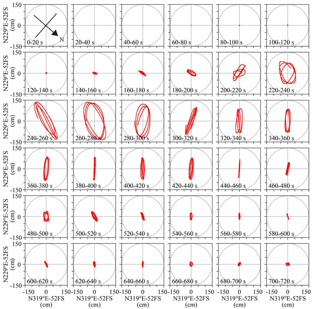
**Figure 5.** Lissajous curves of displacements on the 52nd floor (52FS) of the SKS building
