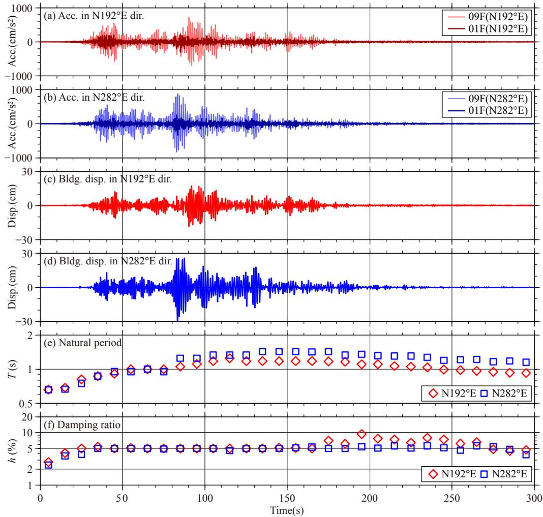
**Figure 2.** Accelerations, building displacements, natural periods and damping ratios of the THU building
