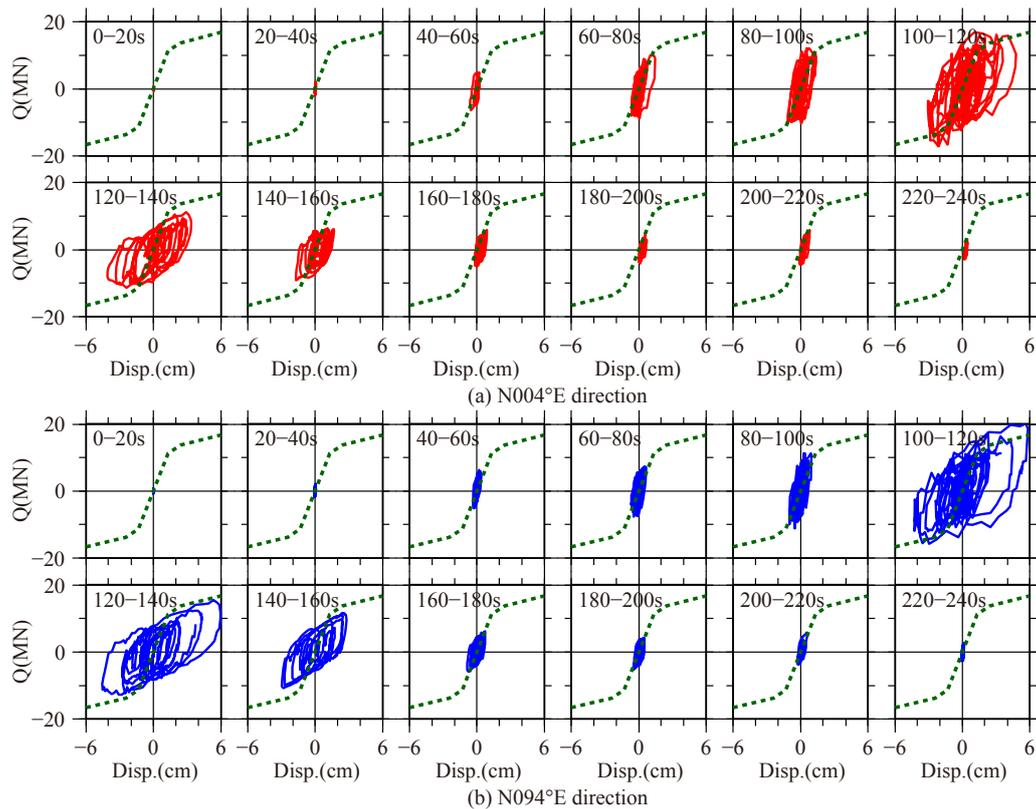
**Figure 7.** Relationship between share force ( $Q$ ) and displacement of the base-isolation devices
