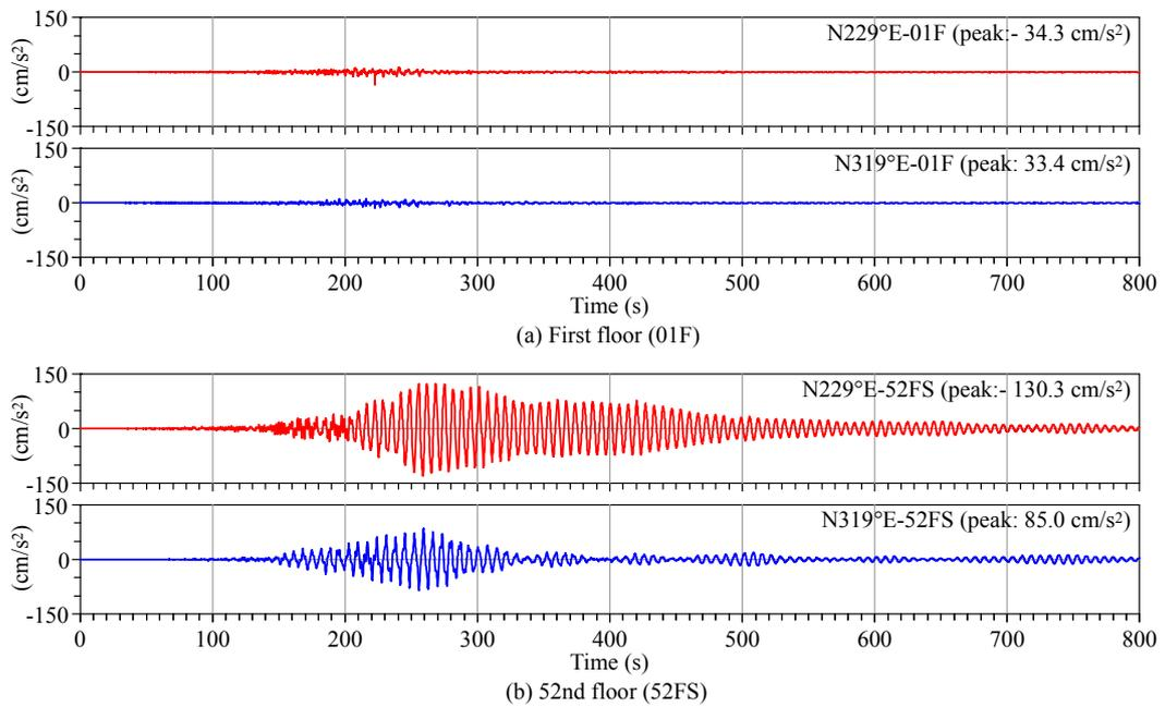
**Figure 3.** Acceleration waveforms on the first floor (01F) and 52nd floor (52FS) at SKS
