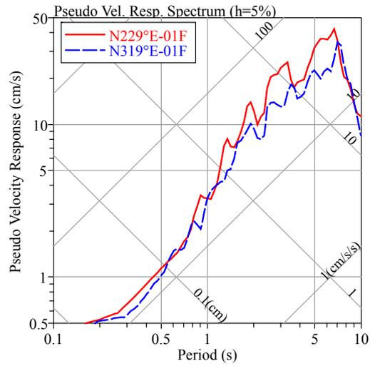
**Figure 4.** Pseudo velocity response spectra of the records on the first floor (01F) of the SKS building
