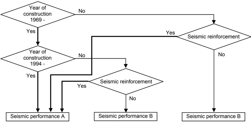
Figure 2. Flow chart of seismic performance classification for bridge structure
