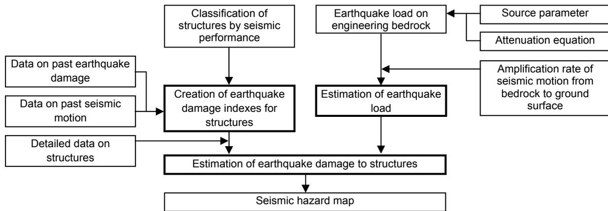
Figure 1. Algorithm for seismic hazard map creation
