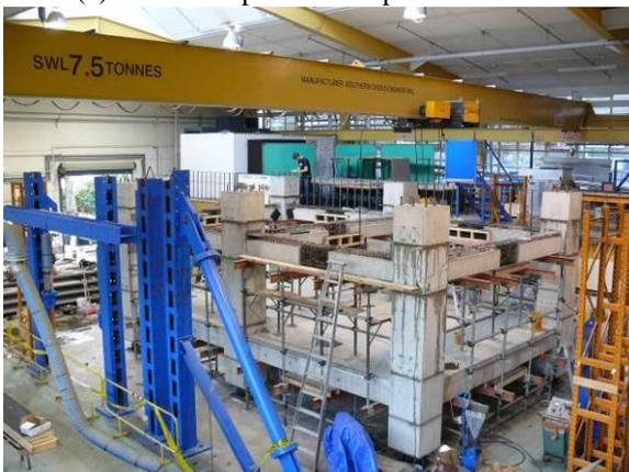
(c) Second floor precast components being grouted.
