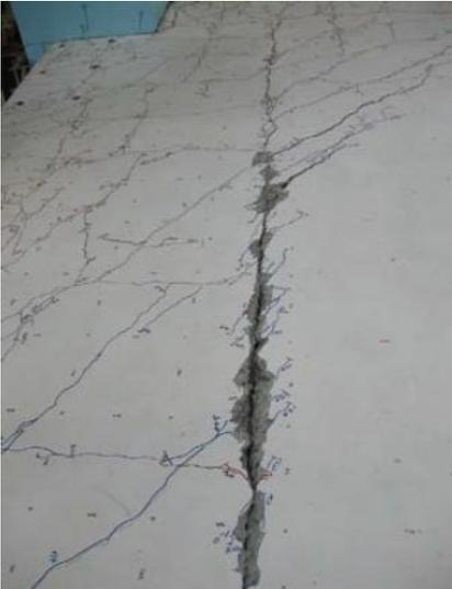
(d) Timber infill cracks, approximately 8mm (Lindsay, 2004).
