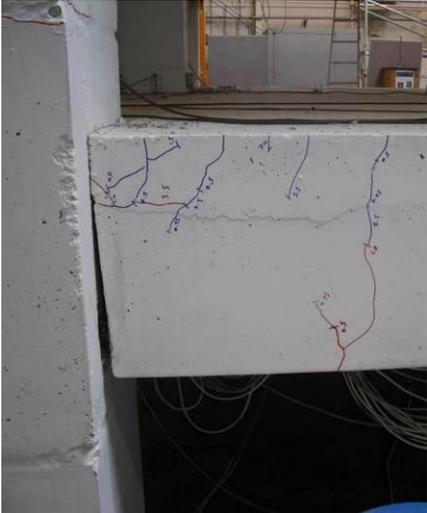
(a) Slotted beam end damage.
