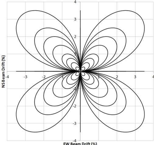
**Figure 2.1.** Combined uniaxial and biaxial displacement protocol.
