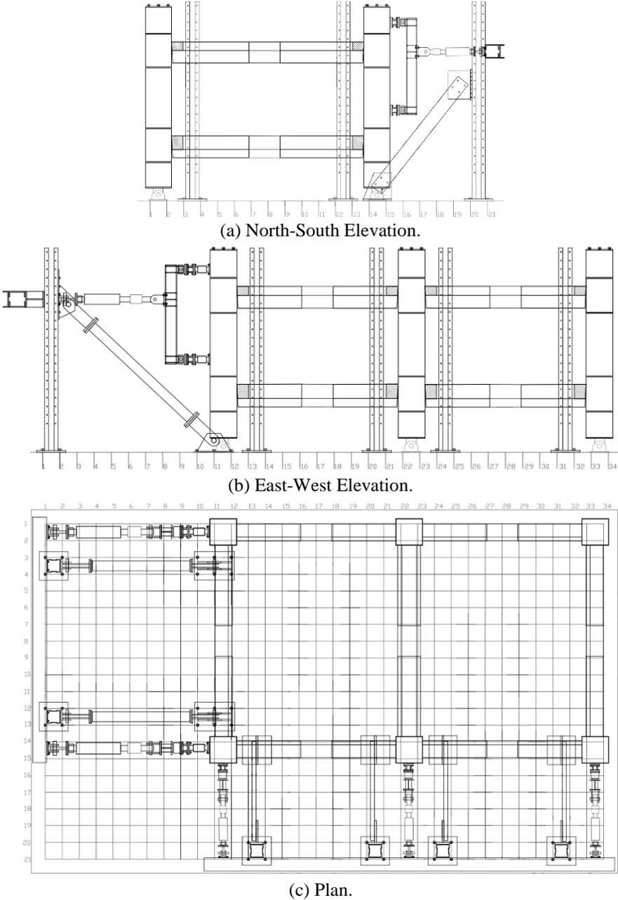
Figure 2.3. Experimental setup drawings.
