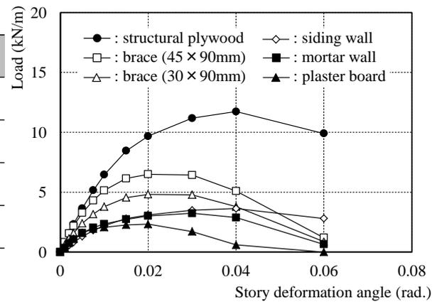
**Figure 2.5.** Skelton curves using the analysis
