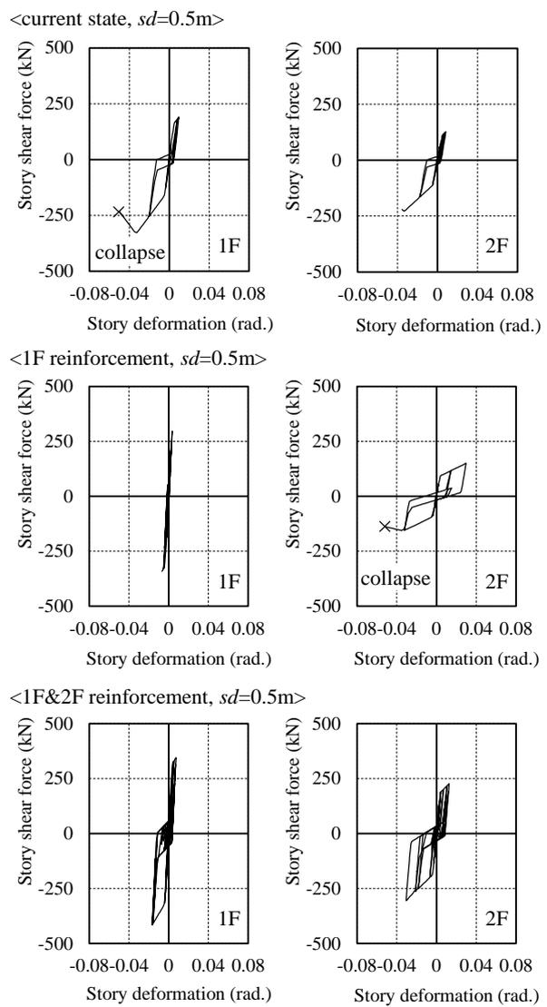
Figure 3.2. Story deformation angle and shear force
