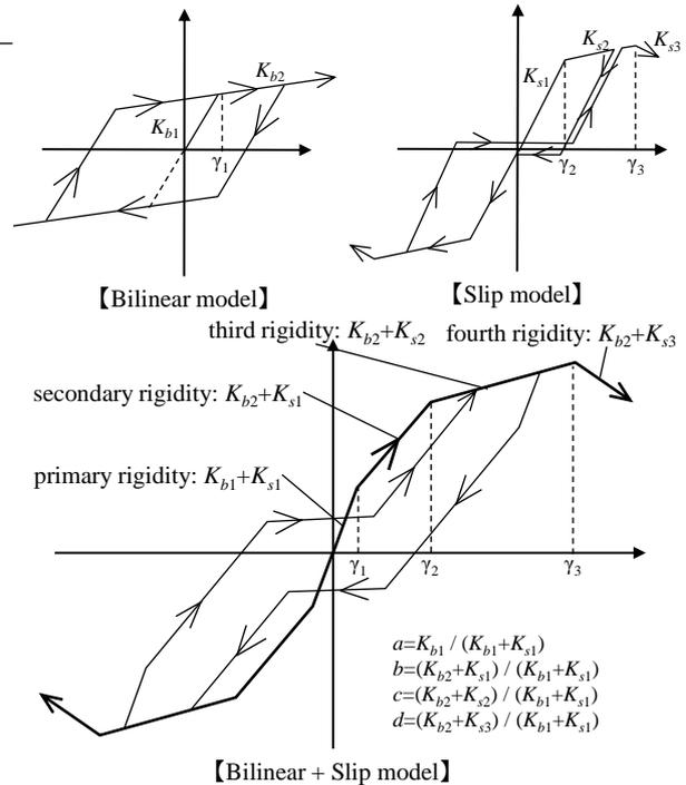
**Figure 2.6.** Analysis models of the structure
