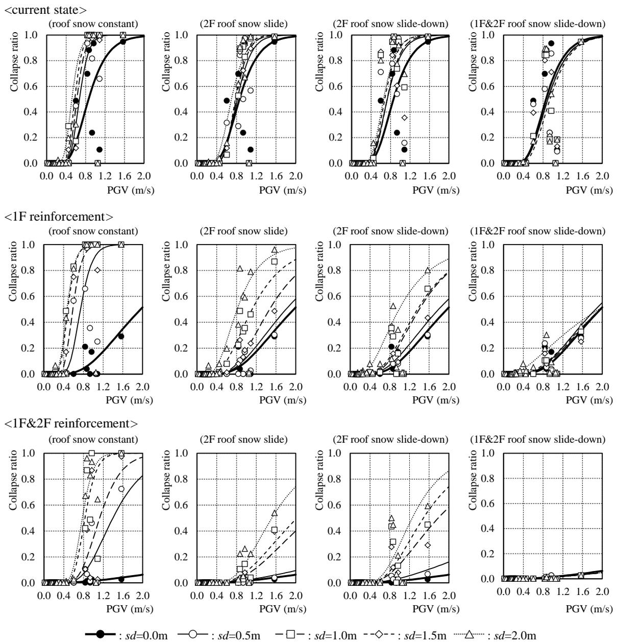
Figure 3.3. Seismic fragility curves in each the reinforcement and dynamic behavior
