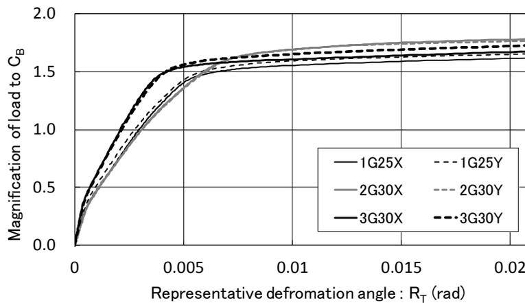
Figure 7. Relationship between base shear coefficient and representative deformation angle
