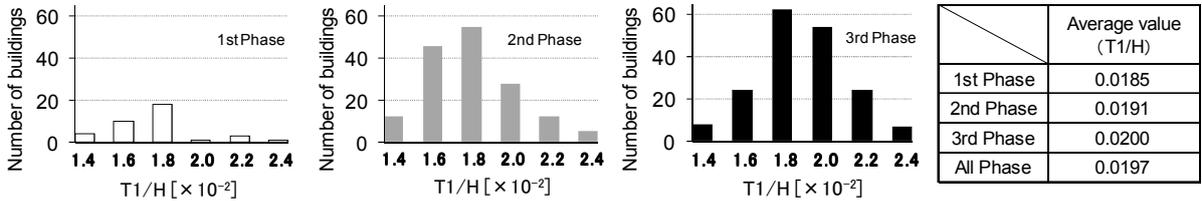
Figure 2. Distribution of number of buildings for the coefficient (T1/H) in three design phases
