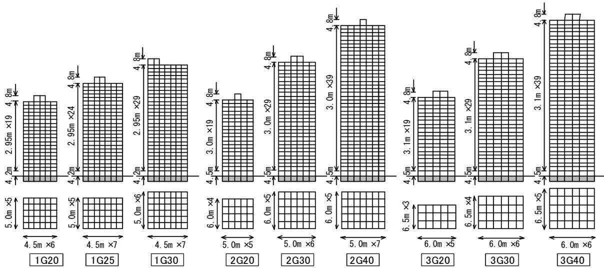
Figure 6. Sketch of framing plan and elevation of framed models
