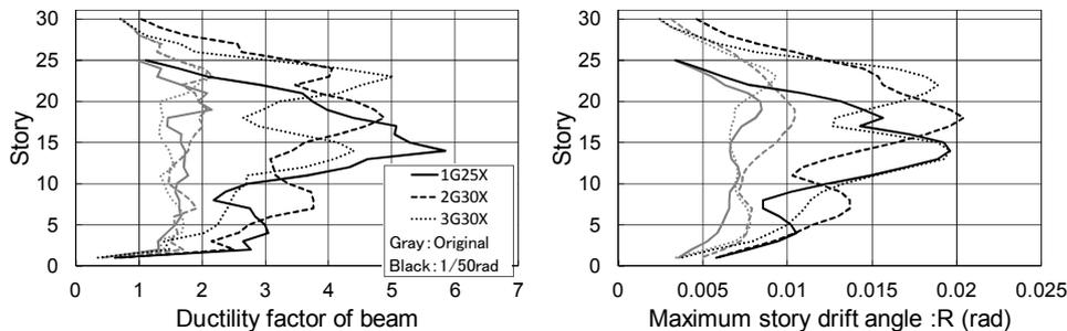
**Figure 11.** Ductility factor of beam and maximum story drift angle
