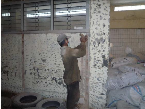
**Photo 2.** Preparation of brick wall specimen
