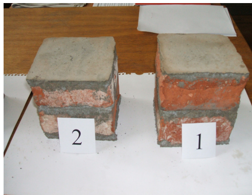
Figure 1. Specimens to determine the compressive strength of pressed full bricks
