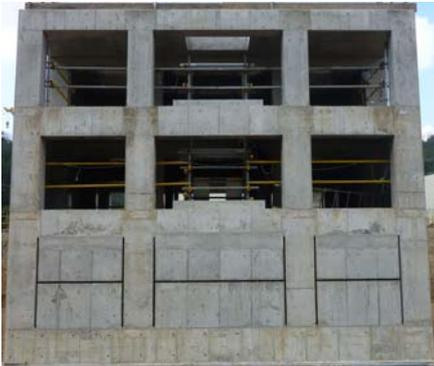
**Photo 2** Building Model and H-shaped Slits in Underground Wall
