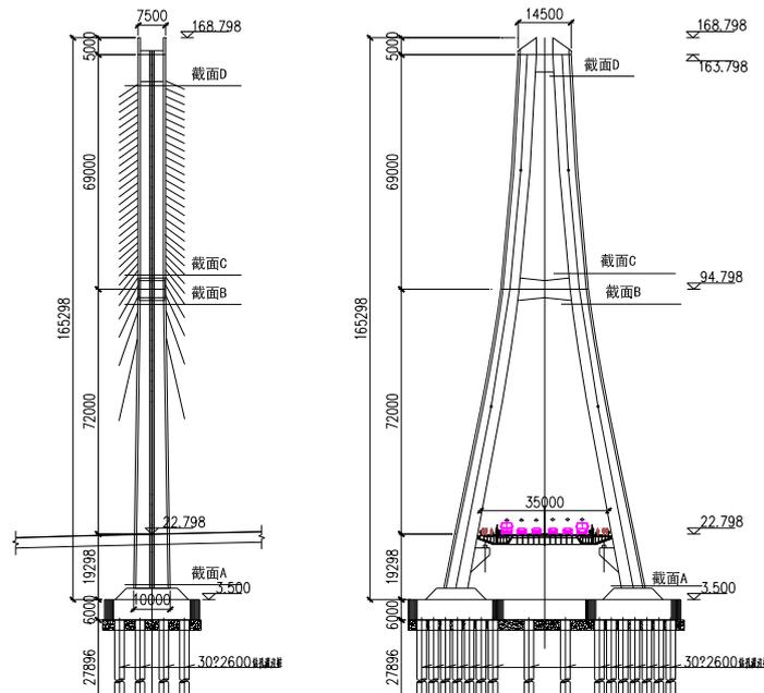
Fig. 2.4 Pylon of the main Bridge (elevation units: m, other units: mm)
