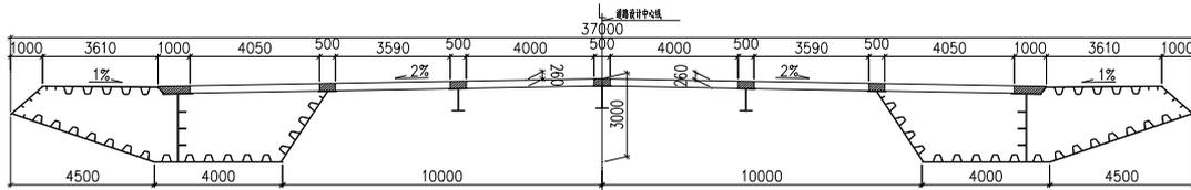
Fig. 2.2 Cross-section of double steel girder (units: mm)
