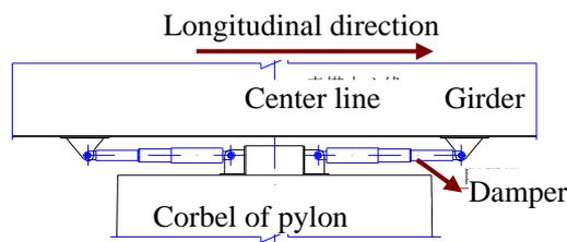
**Fig.6.1** Location of dampers with ultimate stops of the selected design
