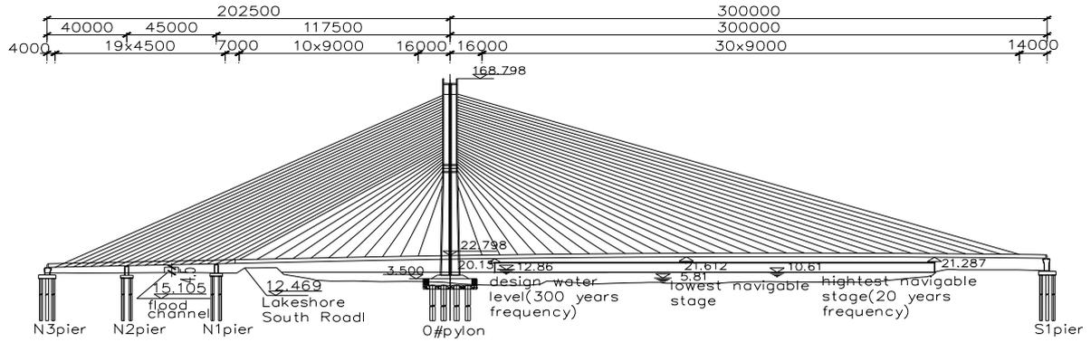
Fig. 2.1 Elevation of the main bridge (elevation units: m, other units: mm)
