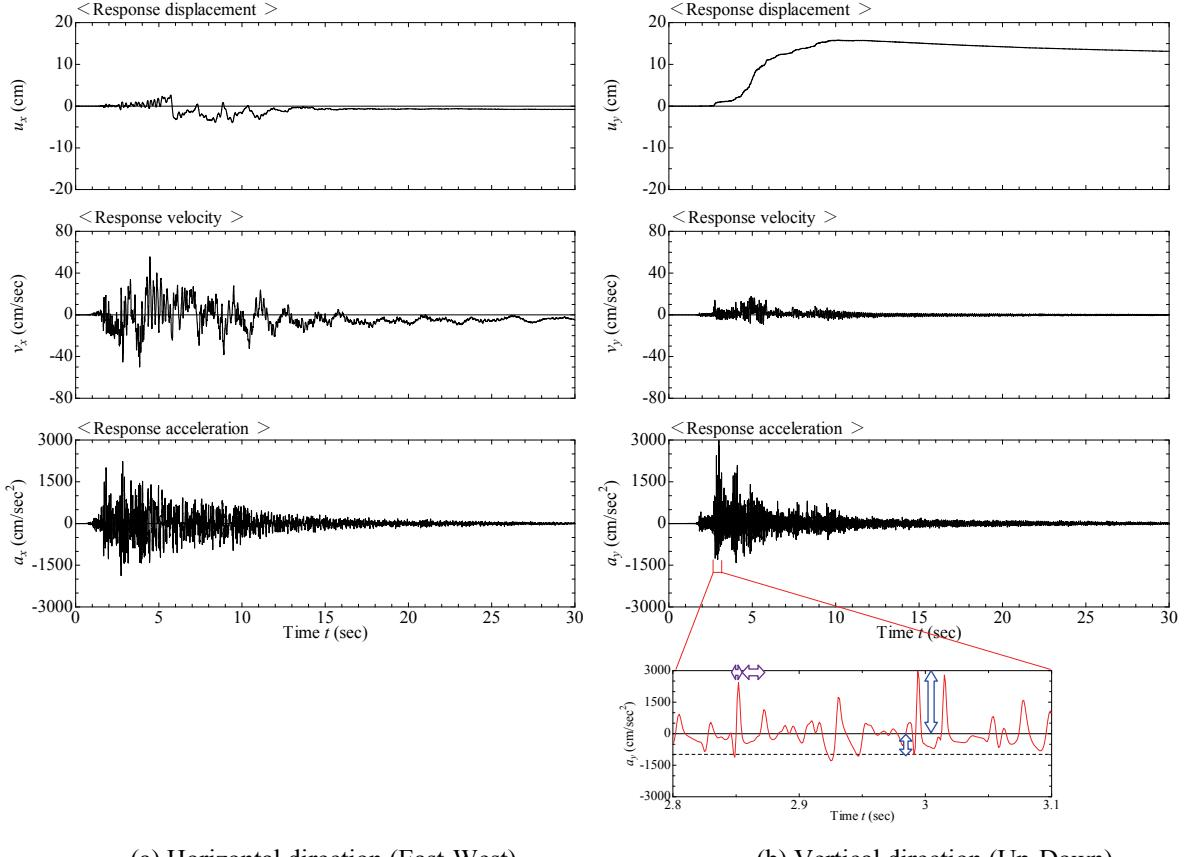
**Figure 6.** Ground surface response (analysis results)
