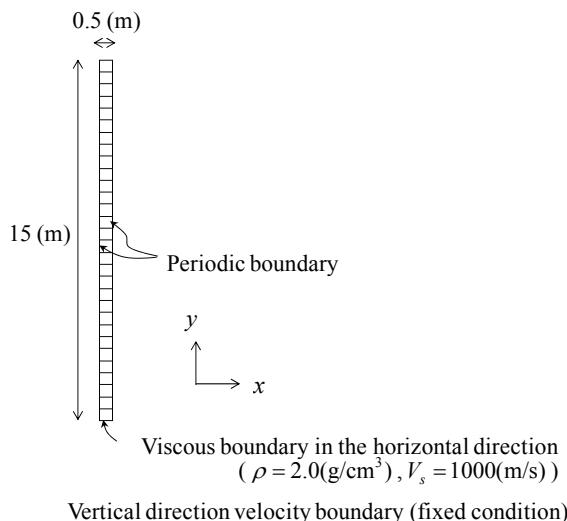
**Figure 2.** Finite element mesh and boundary conditions
