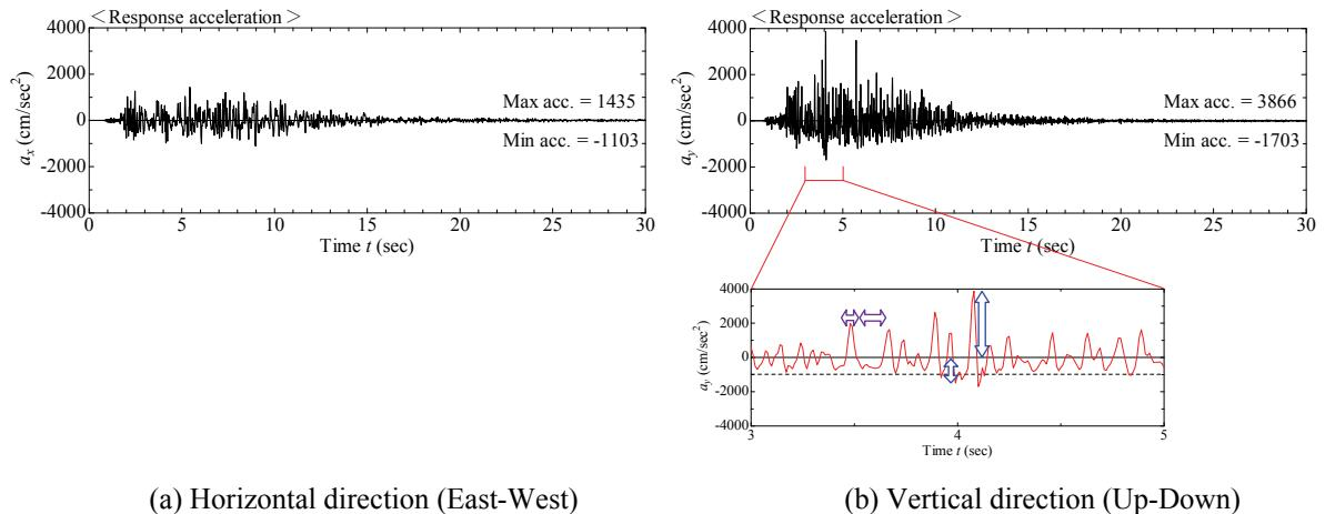
**Figure 5.** Acceleration record measured at the ground surface at KiK-net measurement station IWTH25 (West Ichinoseki)
