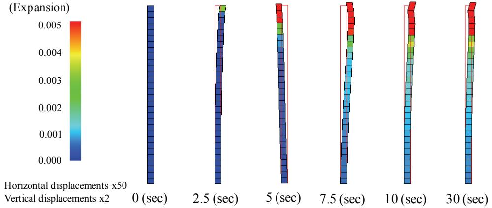
**Figure 7.** Change in distribution of void ratio with time
