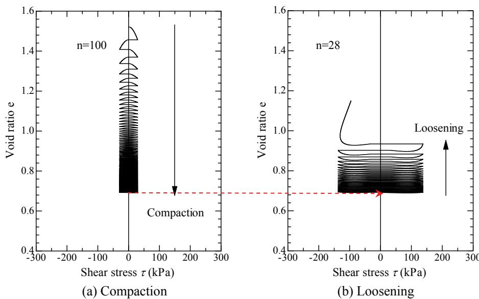
**Figure 1.** Compaction and loosening of soil
