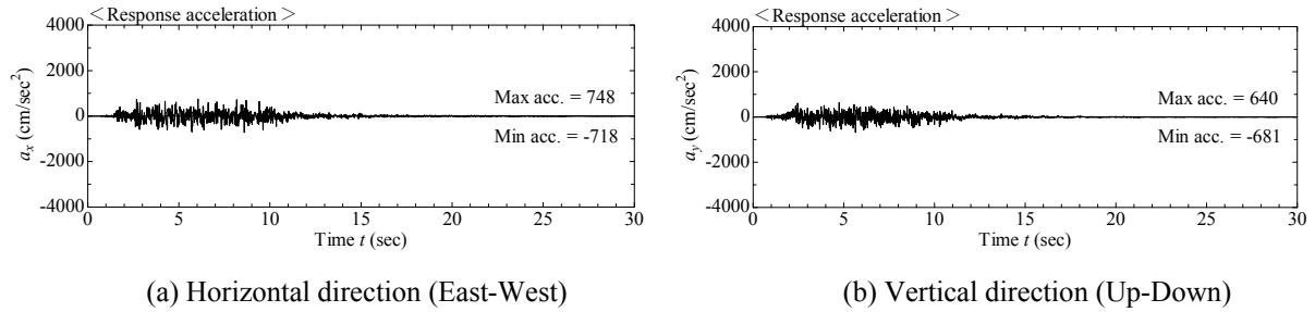
**Figure 4.** Acceleration record measured 260 m below ground at KiK-net measurement station IWTH25 (West Ichinoseki)
