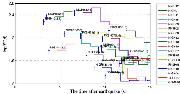
**Figure 3.2** Continual Ground Shaking Prediction using the initial P-wave segments (+for the P-arrival time, Values in brackets for the final value, and lines for the predicted values)
