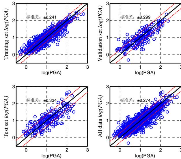
**Figure 2.1** The results of PGA using the ANN within 3s of the P-wave arrival
