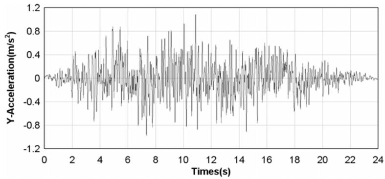
**Figure 4.3.** Time histories of artificial ground motion in streamwise direction
