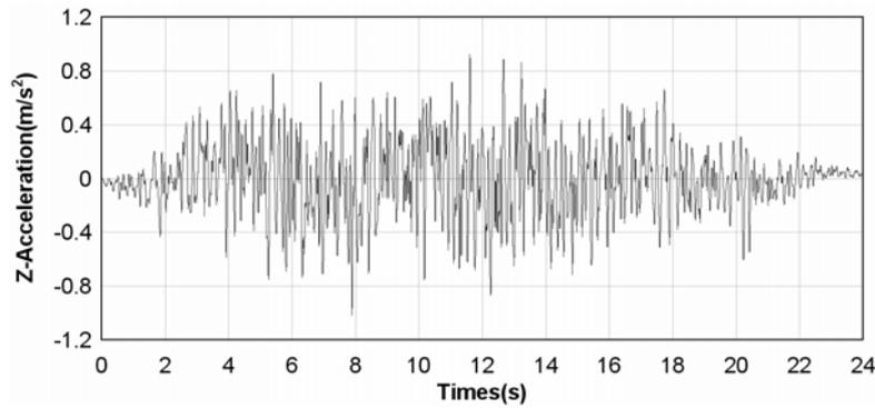
**Figure 4.4.** Time histories of artificial ground motion in vertical direction
