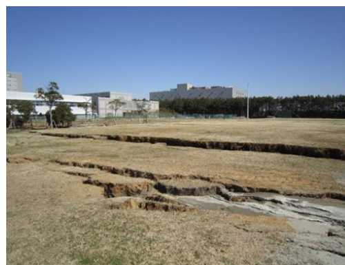
Figure 23. Ground cracks with little sand spread at M2 point
