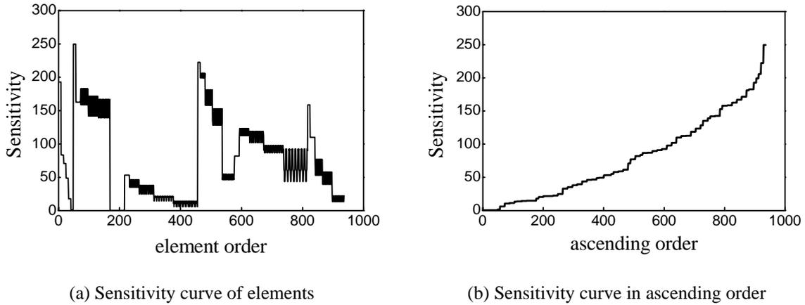
**Figure 5.** Sensitivity generated by section area perturbation of top 20 vibration modes
