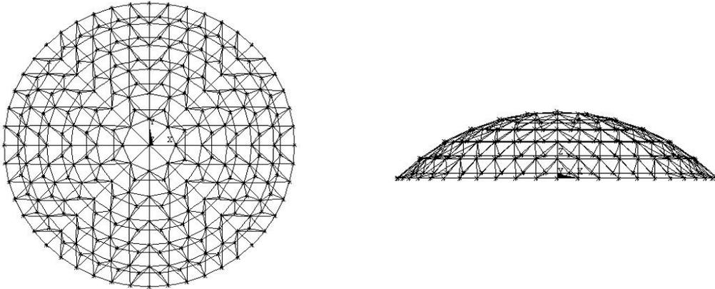
**Figure 1.** Plane and elevation view of double-layer reticulated shell
