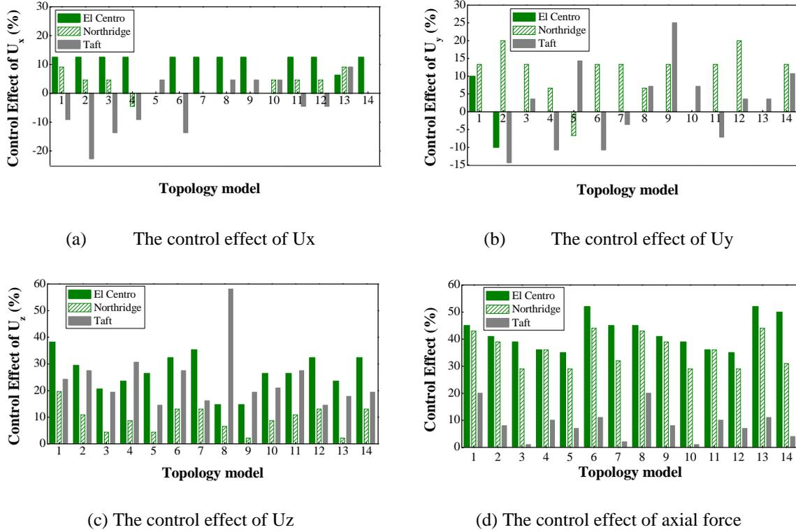
**Figure 4.** Control effect of the maximum displacement of 14 kinds of topologies
