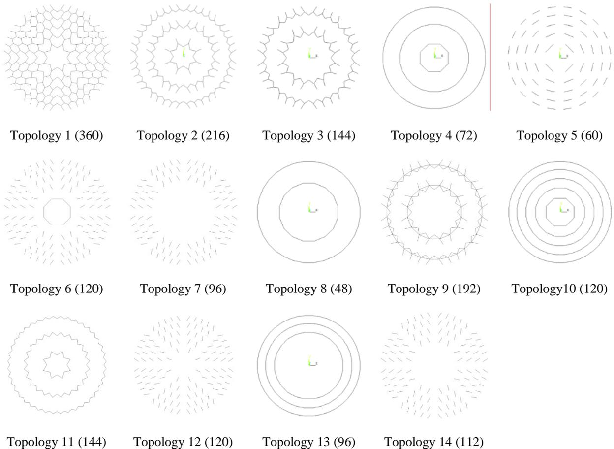
**Figure 3.** Topologies for bar-type VE dampers (The number in brackets is the amount of bar-type dampers)
