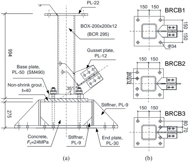
Figure 1. Test specimen: (a) front view; (b) anchor rods layout (unit: mm)
