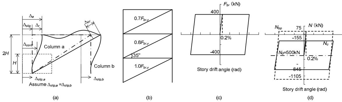
**Figure 3.** (a) Frame deformation; (b) prototype frame; (c) BRB hysteresis behavior; (d) axial force hysteresis behavior
