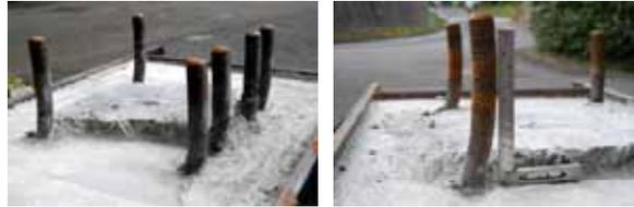
**Figure 4.** Deformation of anchor bolts after the test
