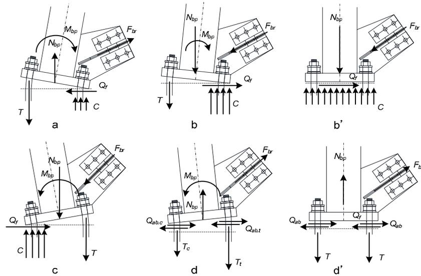
**Figure 7.** Resisting mechanism of column base with BRB
