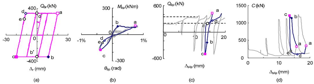
**Figure 6.** (a) Brace behavior; (b) column base slip behavior; (c) column base rotation behavior; and (d)  $C-\Delta_{slip}$  relationship
