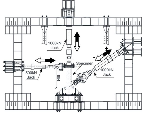
**Figure 2.** Elevation of loading system (unit: mm)
