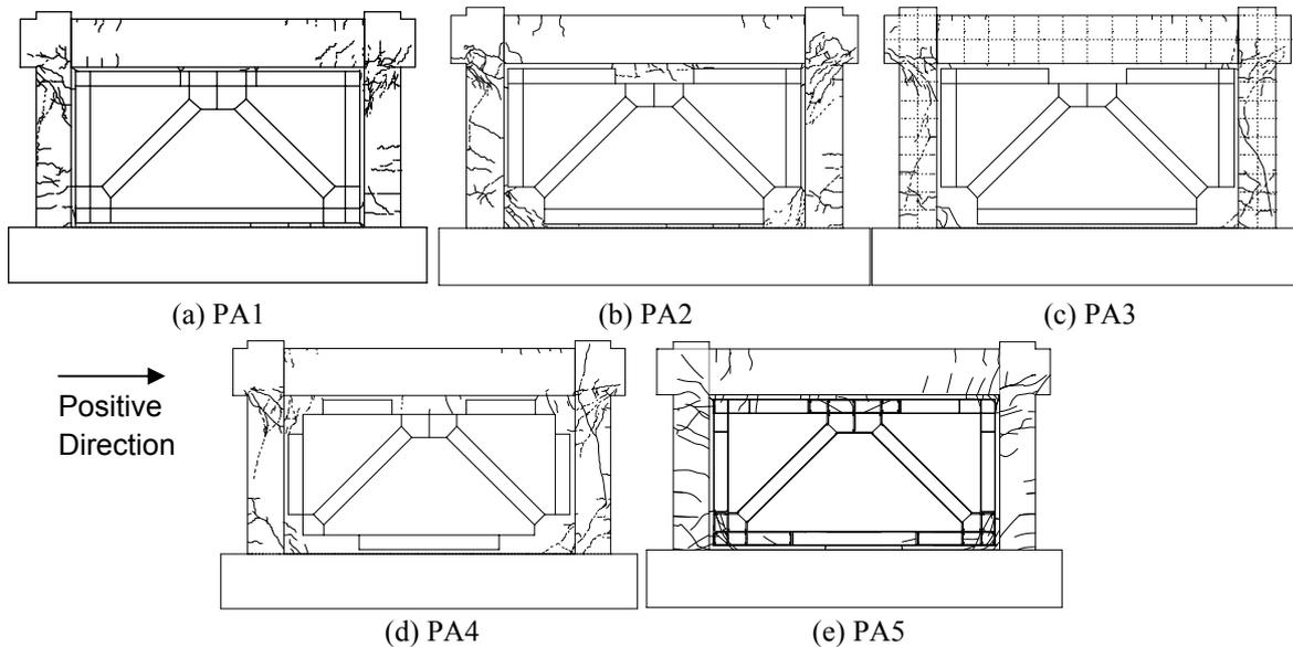
**Figure 4.1.** Crack Patterns at  $R=0.01$ rad.
