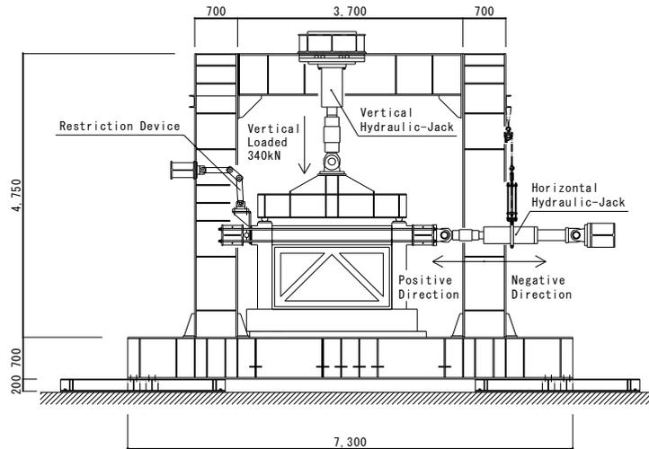
**Figure 3.2.** Loading apparatus
