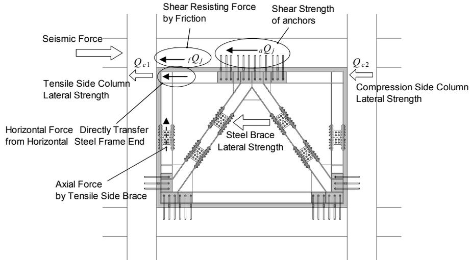
**Figure 5.1.** Horizontal Force Transfer Mechanism
