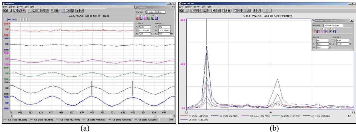
Figure 5.1. Ambient vibration testing. (a) time domain [ $\mu\text{m}$ ]; (b) amplitude Fourier spectra (filter: 0÷2 Hz).
