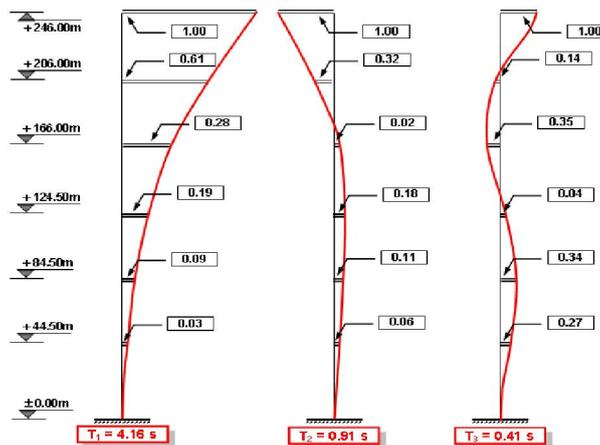
Figure 5.2. Eigenmodes of vibration for the 250 m industrial chimney.
