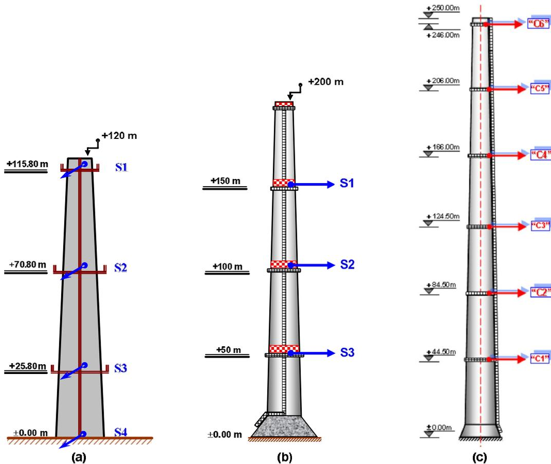
Figure 4.1. Location of sensors in different configurations.
