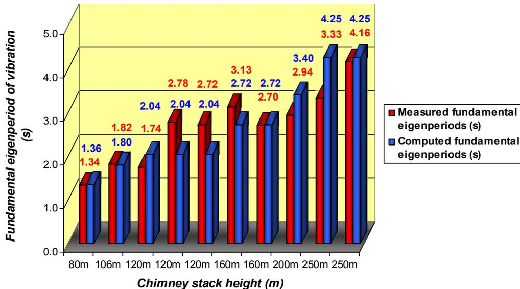
Figure 5.6. Graphic comparison between measured and computed fundamental eigenperiods of vibration.
