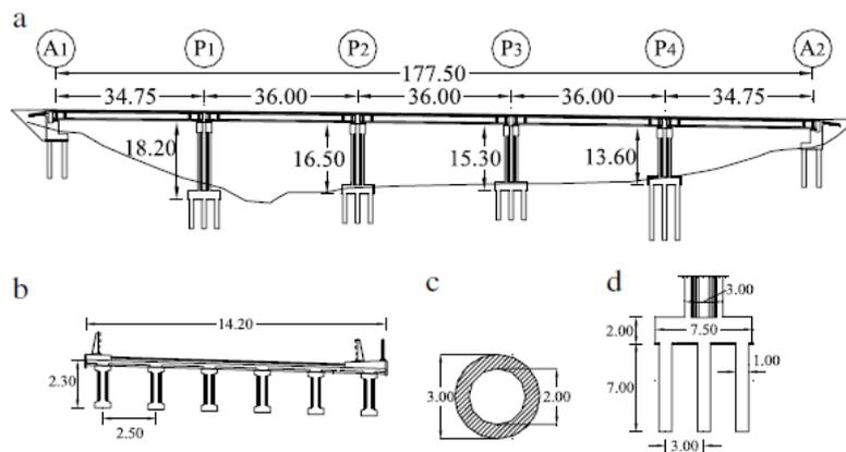
**Figure 6.** (a) Longitudinal section of the simply supported “reference” bridge (b) Deck Cross-section (c) Pier Cross-section (d) Foundation
