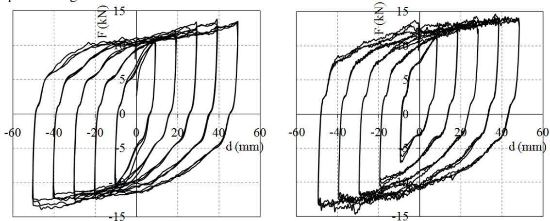
**Figure 11.** Hysteresis loops: (a) slow loading (158mm/min), (b) fast loading (1800mm/min)
