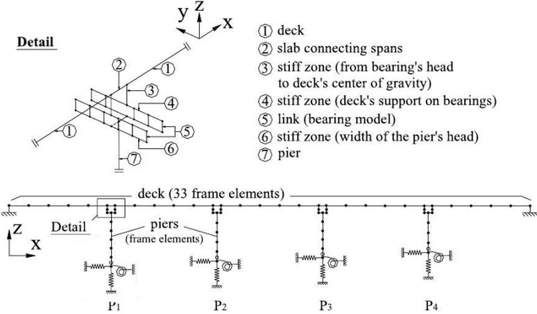
Figure 8. Model of the simply supported bridge
