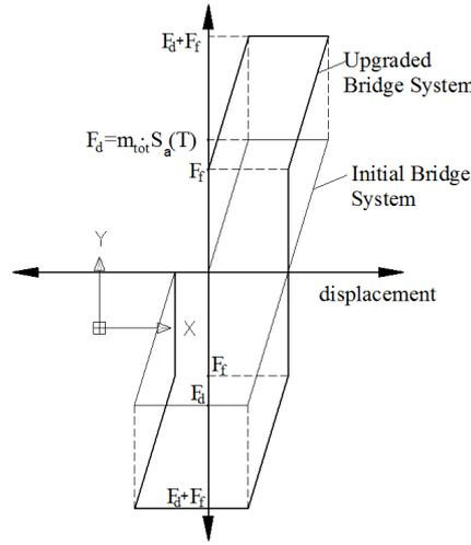
**Figure 4.** Typical hysteresis loops of the initial and the upgraded system
