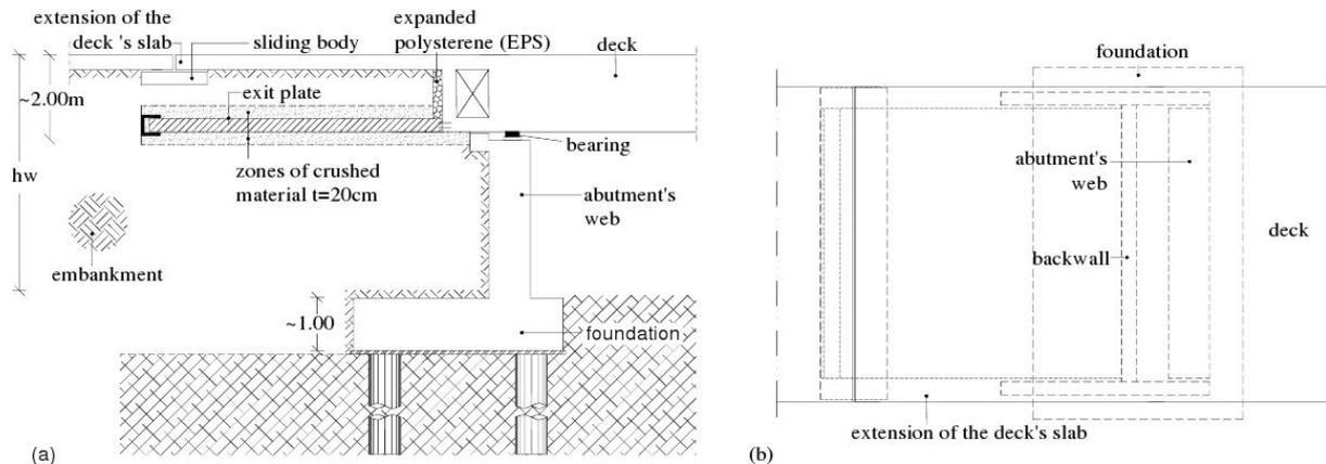
**Figure 3.** The proposed mechanism: (a) longitudinal section and, (b) plan view
