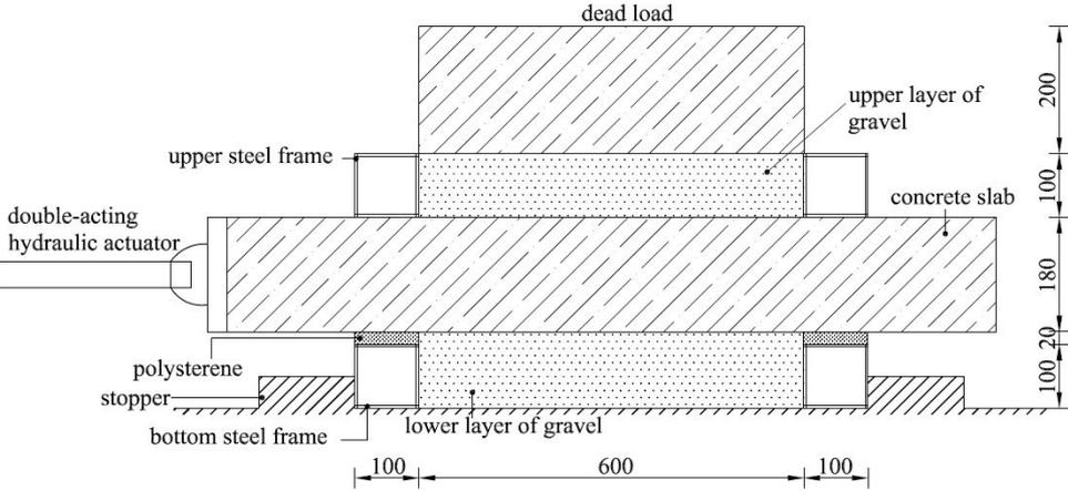
Figure 9. Cross Section of the Experimental Setup
