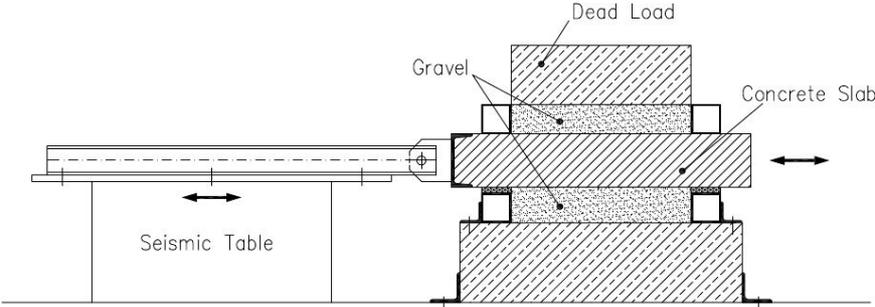
(b) Parametric Study of Soil Type, Frequency, Roughness etc
