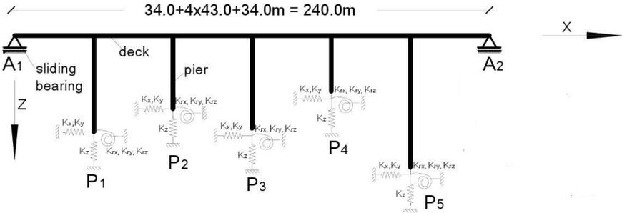
Figure 7. Model of the integral bridge
