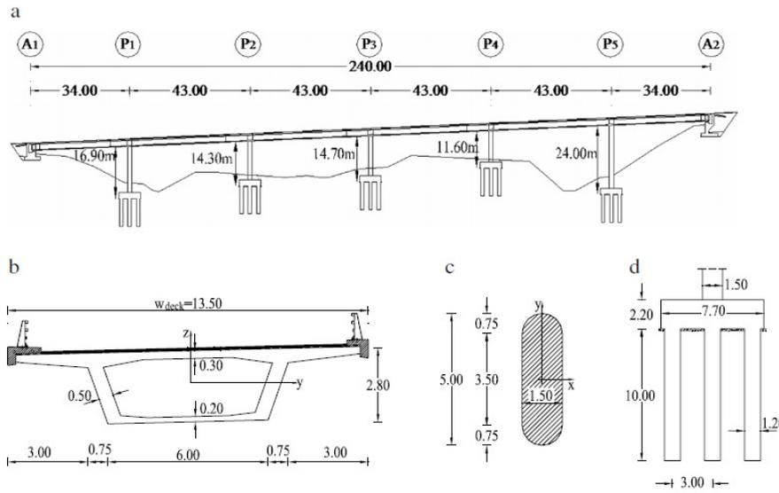
**Figure 5.** (a) Longitudinal section of the integral “reference” bridge (b) Deck Cross-section (c) Pier Cross-section (d) Foundation
