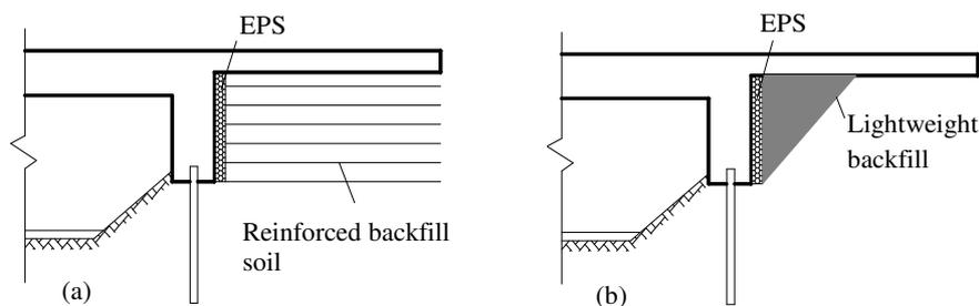
**Figure 1.** Structural techniques proposed by Horvath for the minimization of the ratcheting effect in US bridges: (a) reinforced backfill and (b) lightweight backfill
