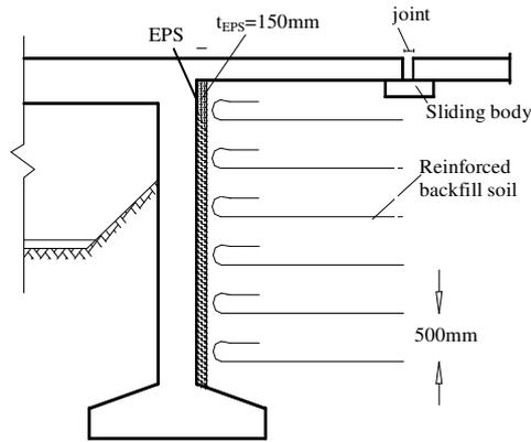
**Figure 2.** Compressible inclusion (EPS) between the reinforced backfill and the full height abutment (Germany)
