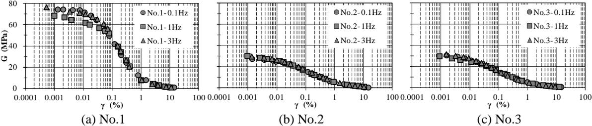
Figure 3. Shear modulus vs. shear strain
