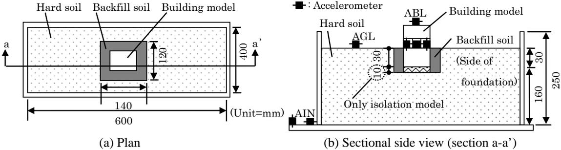
Figure 5. Plan and sectional side view of the experimental model
