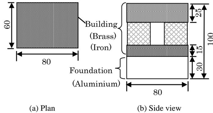
**Figure 6.** Plan and side view of building model
