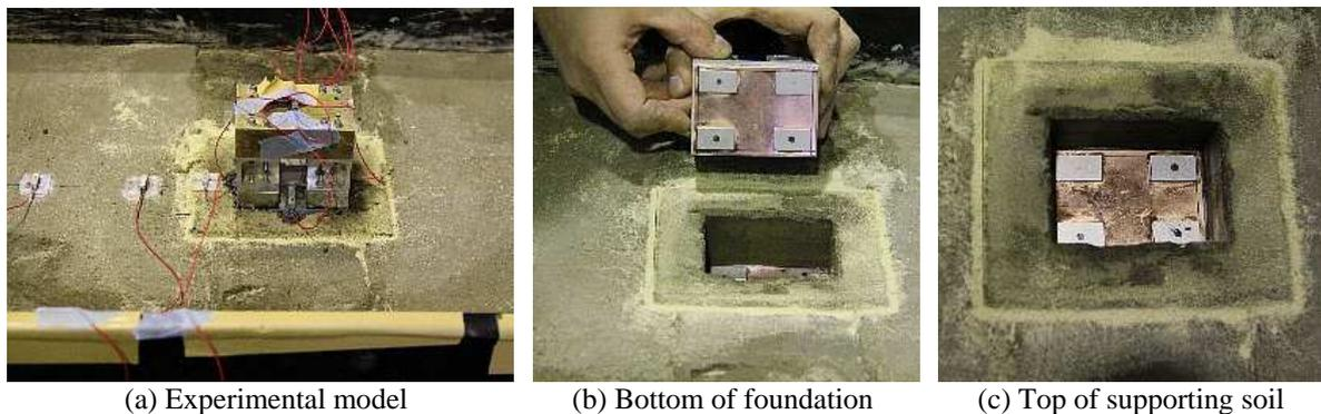
**Photograph 2.** Experimental model and neodymium magnets attached
