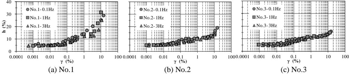
Figure 4. Damping ratio vs. shear strain
