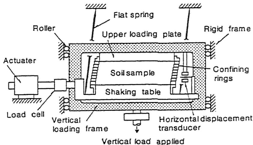
Figure 1. Schematic view of cyclic simple shear testing apparatus
