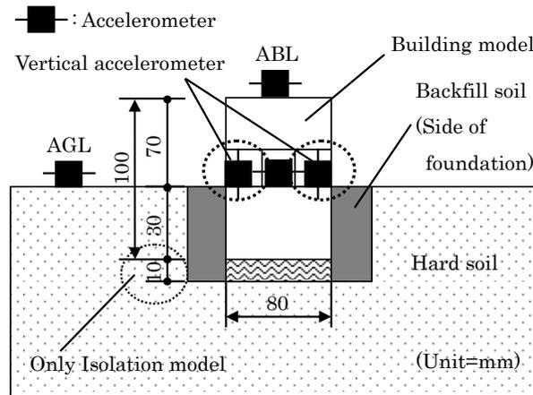
**Figure 11.** Accelerometer layout sketch
