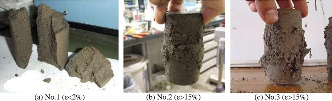
Photograph 2. Failure conditions of specimens after unconfined compression test
