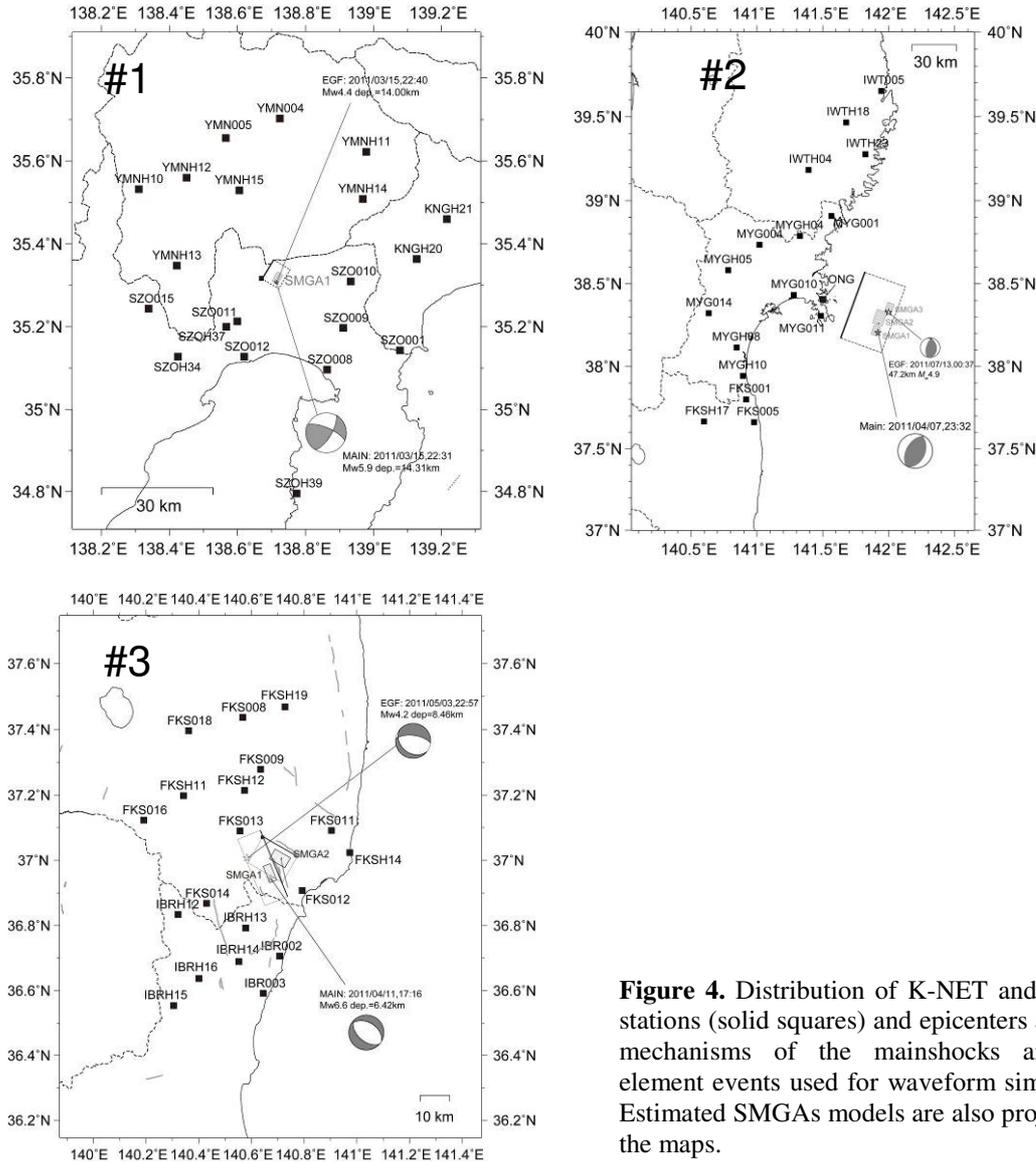
**Figure 4.** Distribution of K-NET and KiK-net stations (solid squares) and epicenters and focal mechanisms of the mainshocks and EGF element events used for waveform simulations. Estimated SMGAs models are also projected on the maps.
