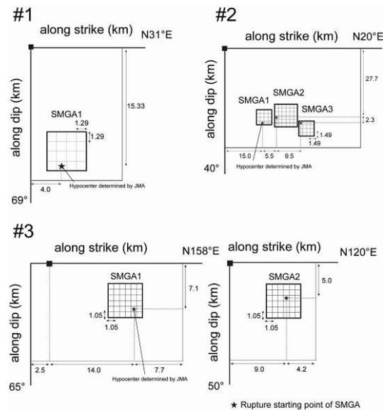
**Figure 5.** Source models of each earthquake. The star indicates the rupture starting point of each SMGA.
