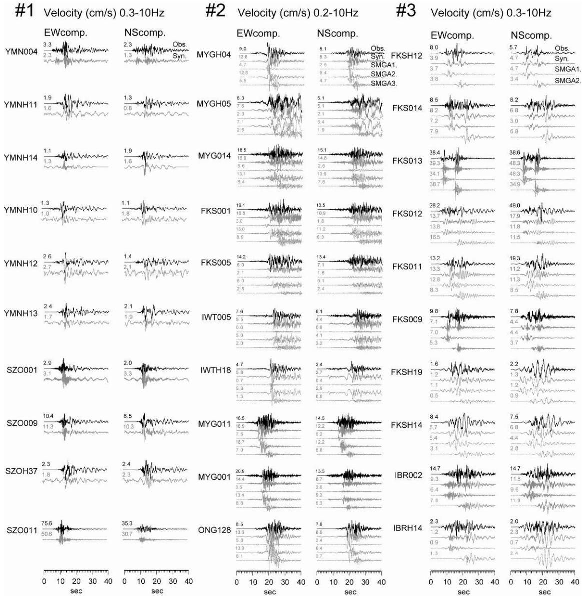
**Figure 6.** Examples of Comparisons among observed velocity waveforms (solid black line), synthetic waveforms (solid gray line) and synthetic waveforms generated from each SMGA (dashed gray line). The two horizontal components are shown. Number indicates the maximum amplitude of each velocity waveforms in cm/s.
