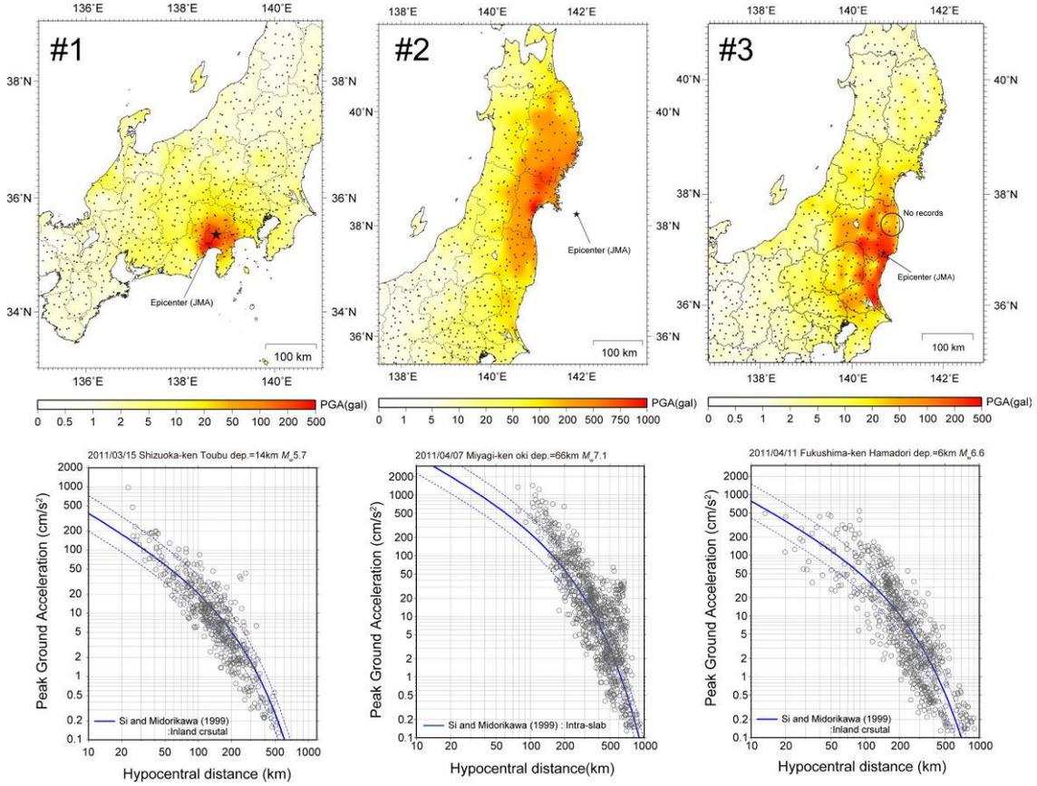
**Figure 3.** Top: Spatial distribution of peak ground acceleration (PGA) from each induced earthquake. The star is the epicenter of each event. Black dots indicate K-NET and KiK-net stations. Bottom: Distribution of PGA values over distance. The empirical relationship (solid curve) and standard deviations (dashed curves) proposed by Si and Midorikawa (1999) are also shown.
