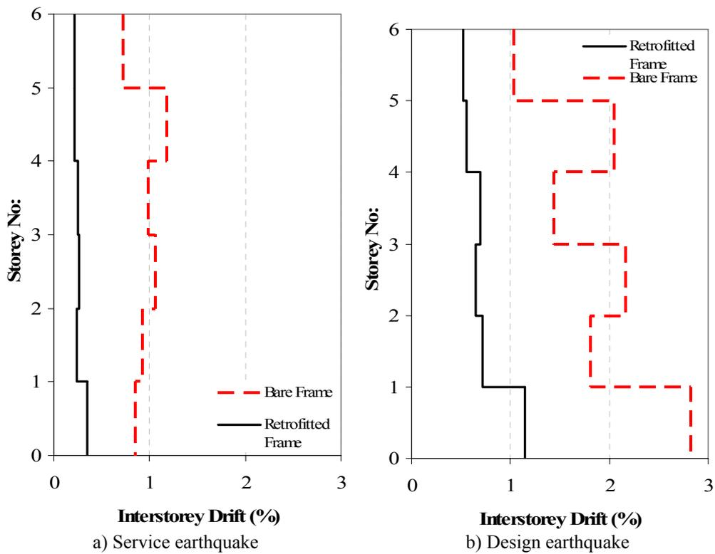
**Figure 10:** Comparison of the maximum interstorey drift of the frame with and without shotcrete panel for “service” and “design” earthquakes
