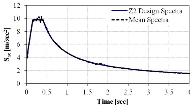
Figure 8: Design spectrum defined in TEC, 2007
