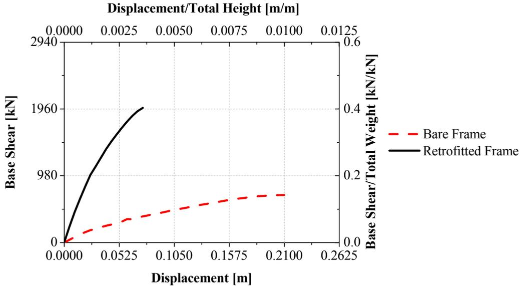
**Figure 4:** Base shear-top displacement and base shear/total weight-top displacement/total height diagram
