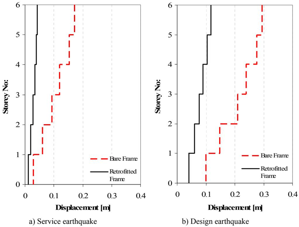
**Figure 9:** Comparison of the maximum story displacements of the frame with and without shotcrete panel for “service” and “design” earthquakes
