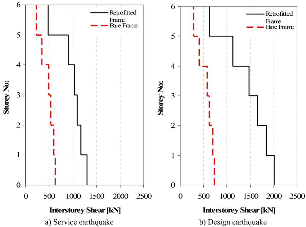
**Figure 11:** Comparison of the maximum interstorey shear force of the frame with and without shotcrete panel for “service” and “design” earthquakes
