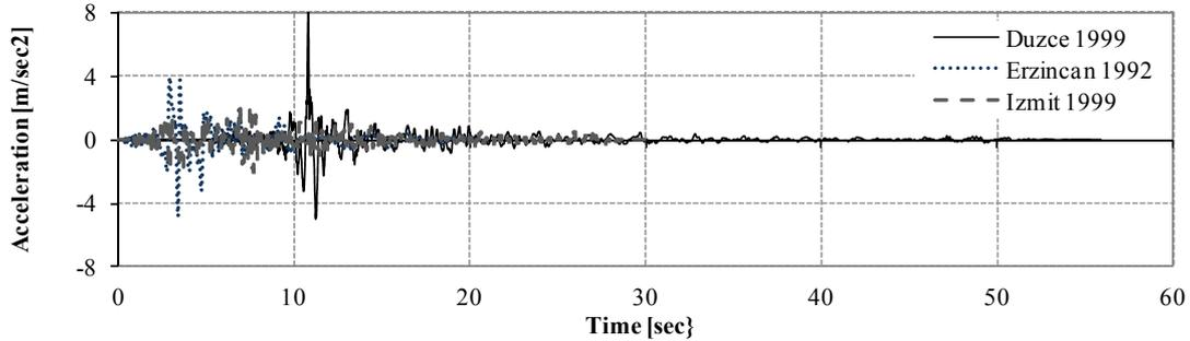
**Figure 5:** The acceleration record of Erzincan, İzmit and Düzce Earthquake, PEER (2007)
