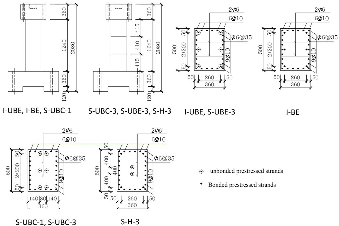
**Figure 2.1.** Specimen details
