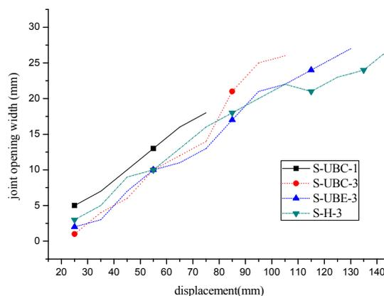
**Figure 3.10** the joint opening width - displacement
