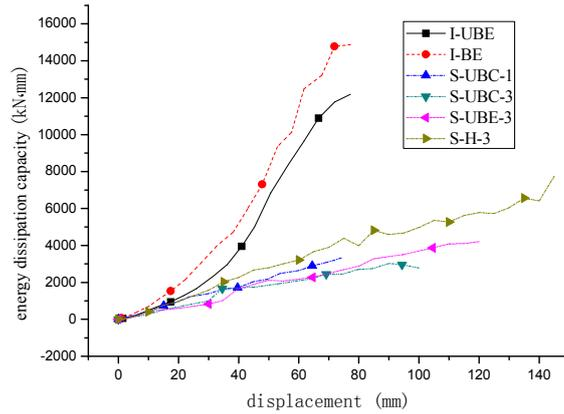
**Figure 3.8** Energy dissipation capacity-displacement curve
