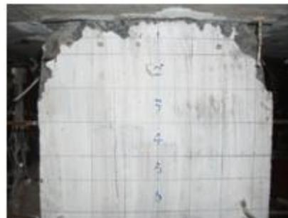
**Figure 3.3** The angle of the joint opening **Figure 3.4** Observed failure mode of specimen S-UBE-3
