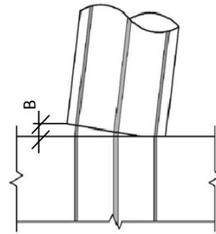
**Figure 3.1** Observed failure mode of specimen I-UBE **Figure 3.2** Segmental specimen joint deformation form
