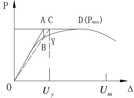
**Figure 3.6** The envelope of cyclic load-displacement curve **Figure 3.7** Definition of displacement ductility
