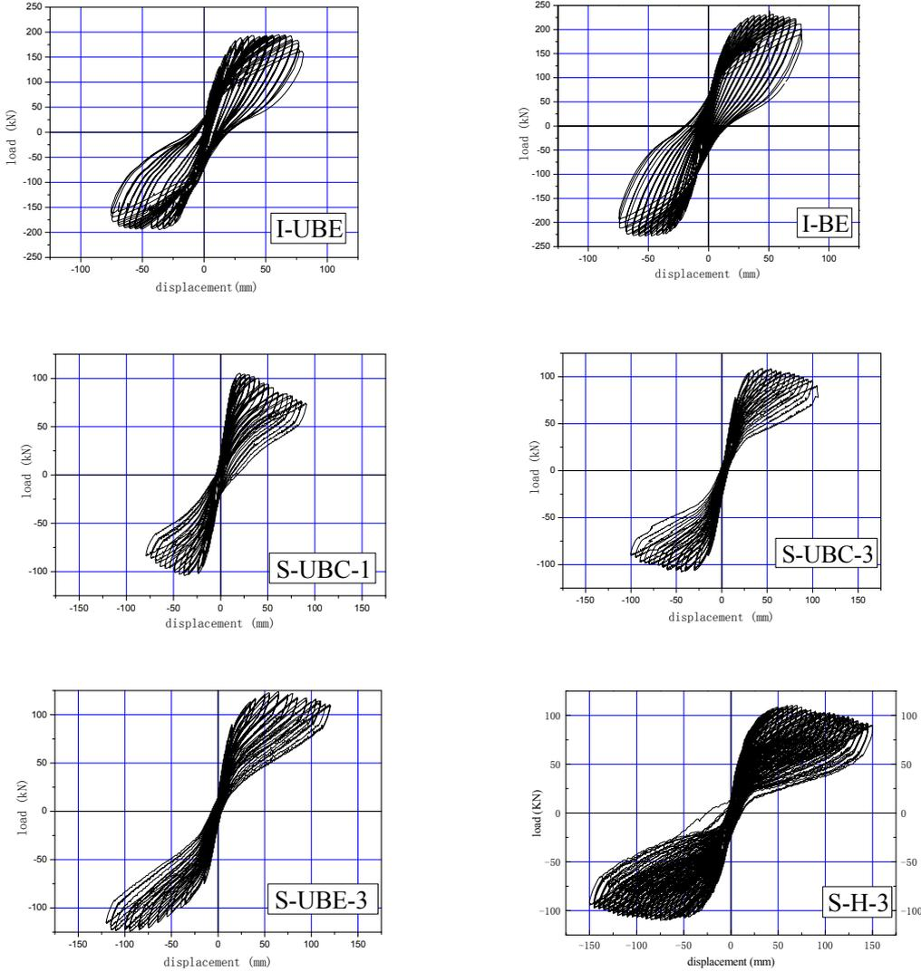
**Figure 3.5** Load-displacement hysteretic curves of specimens
