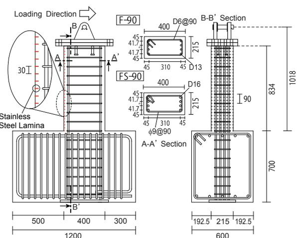
**Figure 2.** Dimension of beam specimen (F-90/FS-90)
