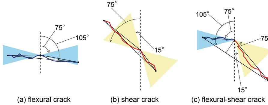
**Figure 14.** Crack type definition due to its growth angle
