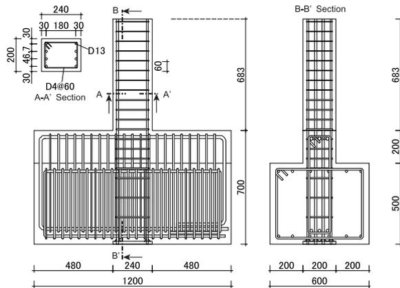
**Figure 8.** Dimension of beam specimen
