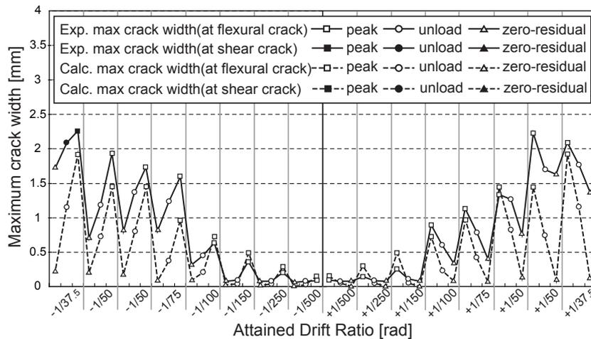
**Figure 20.** Crack width estimation of specimen F-1
