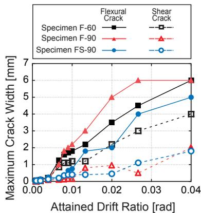
**Figure 6.** Crack width for attained drift ratio
