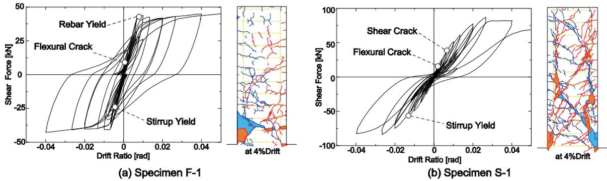
**Figure 11.** Shear force versus drift ratio response, and cracking pattern
