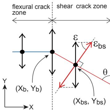
**Figure 15.** Inflection point and converted strain  $\varepsilon_{bs}$
