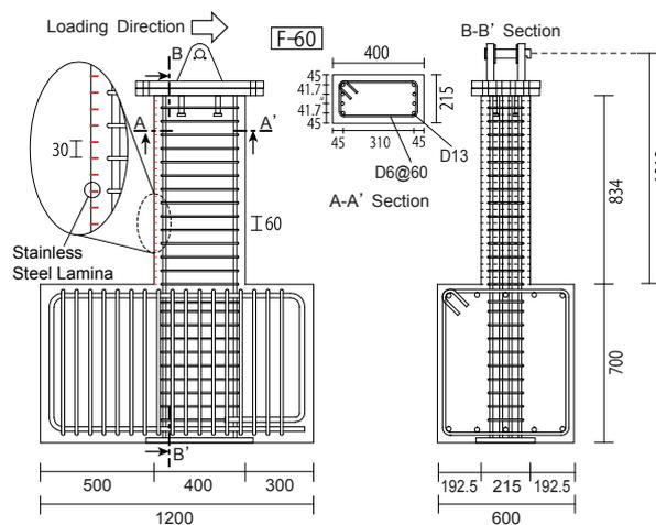
**Figure 1.** Dimension of beam specimen (F-60)
