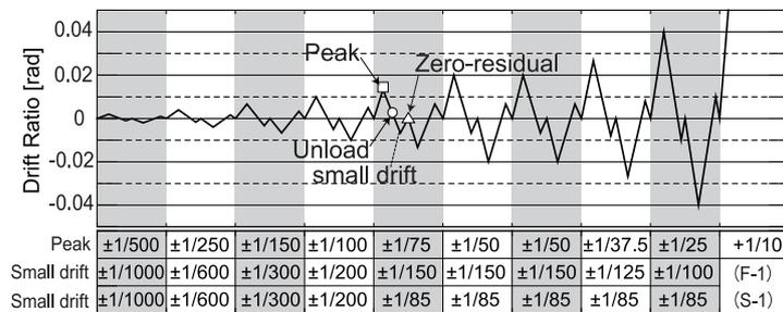
**Figure 10.** Cyclic displacement pattern
