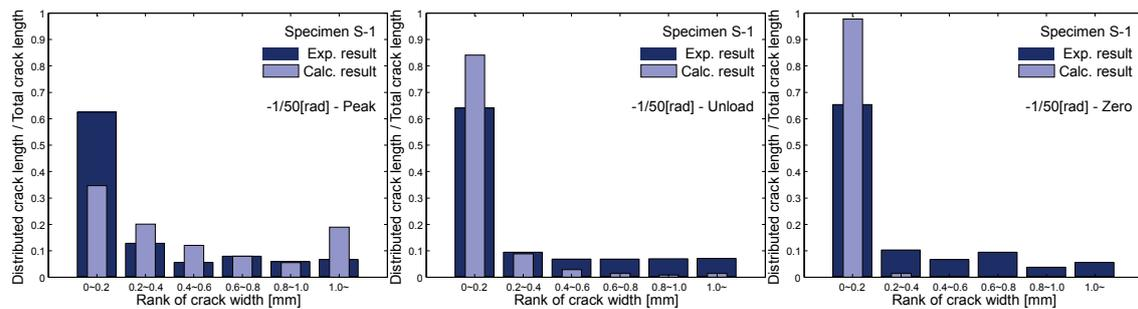
(b) Specimen S-1 at the attained drift ratio = 0.02 rad.
