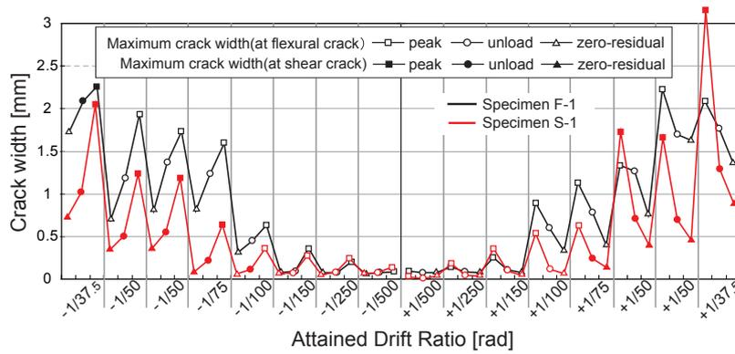
**Figure 12.** Crack width for attained drift ratio
