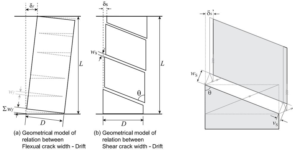
**Figure 18.** Geometrical model of crack width and drift **Figure 19.** Shear crack width and drift
