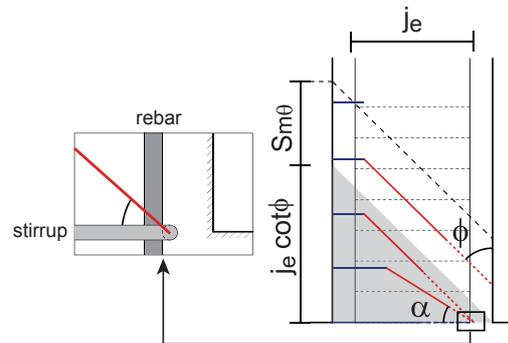
**Figure 16.** Orientation of crack propagation
