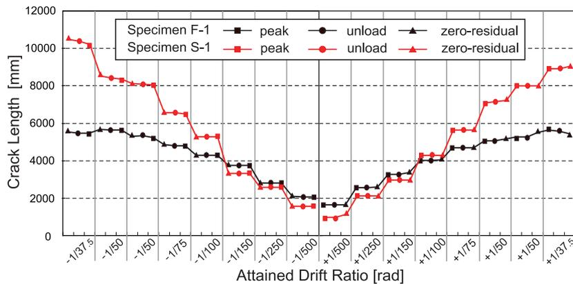
**Figure 13.** Crack length for attained drift ratio
