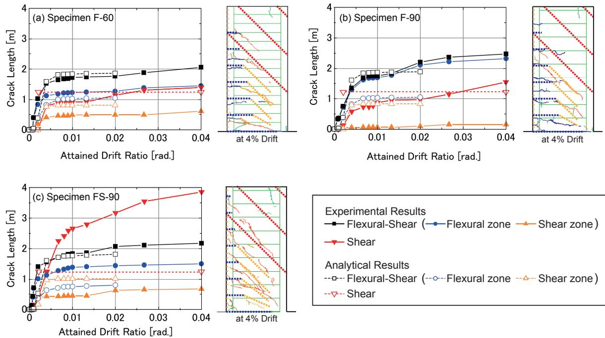
Figure 17. Comparison between the estimated crack length and experimental result
