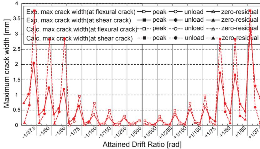
Figure 21. Crack width estimation of specimen S-1
