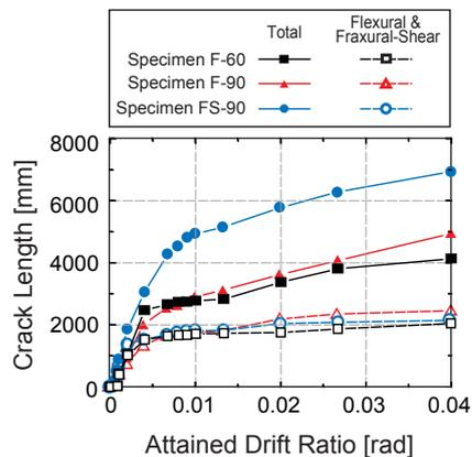
**Figure 7.** Crack length for attained drift ratio
