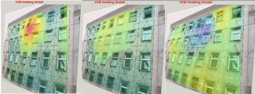
**Figure 5:** Vibration behavior in the reference measurement at an excitement frequency of 11,75 Hz
