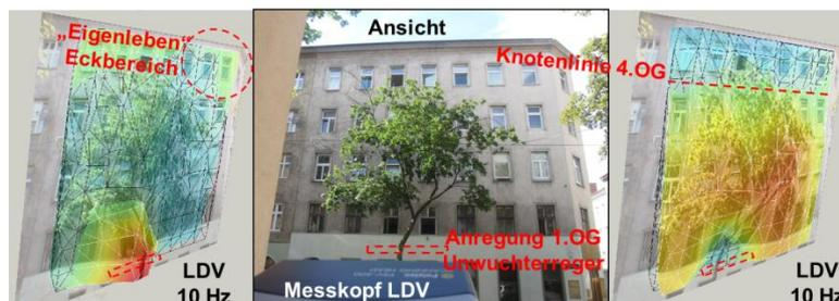
**Figure 2:** Result of a measurement of a facade, which has been excited harmonically in the 1st floor
