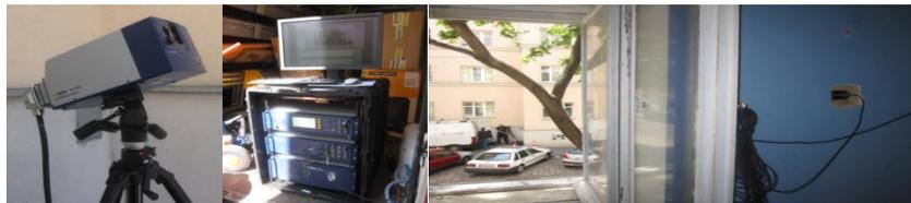
**Figure 1:** Laser-Doppler-Vibrometer: single measurement position, electronic components, reference sensor
