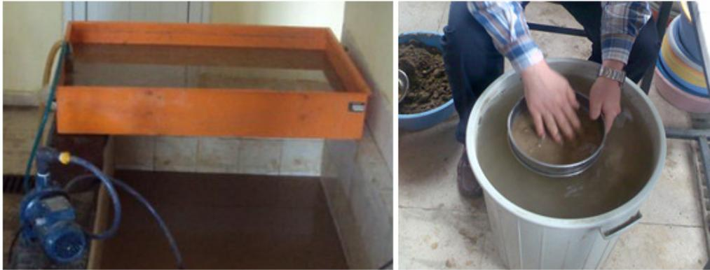
**Figure 1.** a) Removing clay by vacuum      b) Removing sand by washing through No.200 sieve
