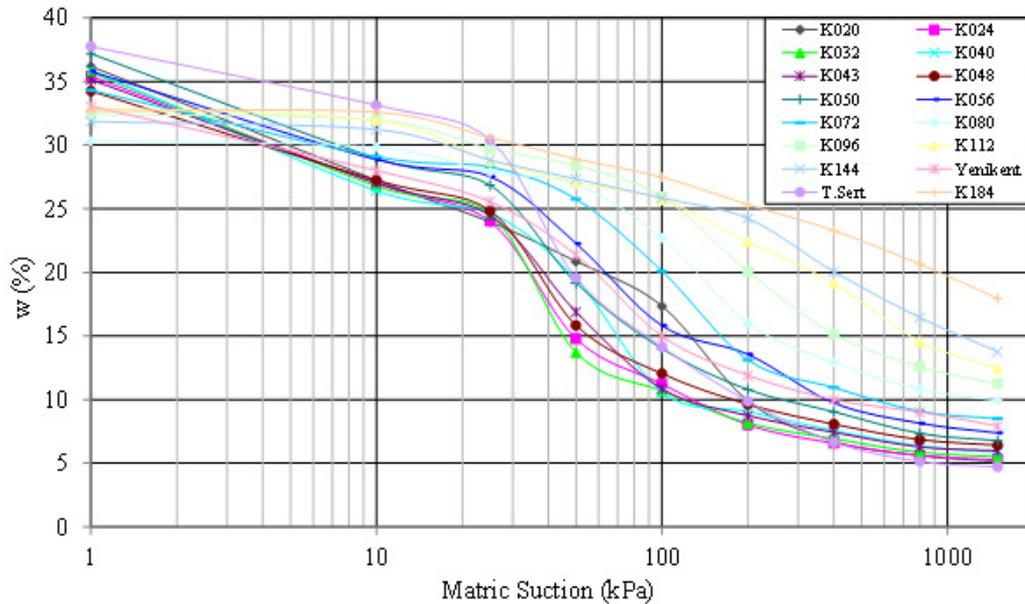
Figure 7. SWCC curves formed by pressure plate tests
