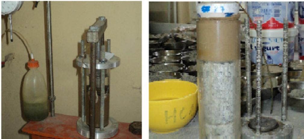
**Figure 2.** Consolidation of the slurry and extraction from the mold
