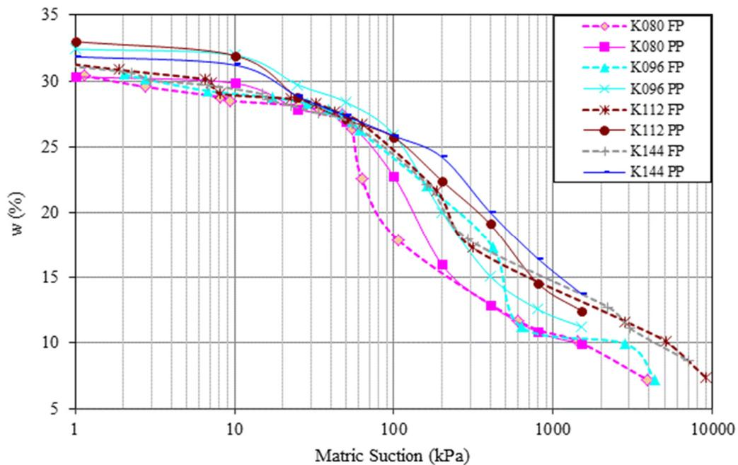
Figure 8. SWCC of four samples formed with both filter paper and pressure plate tests
