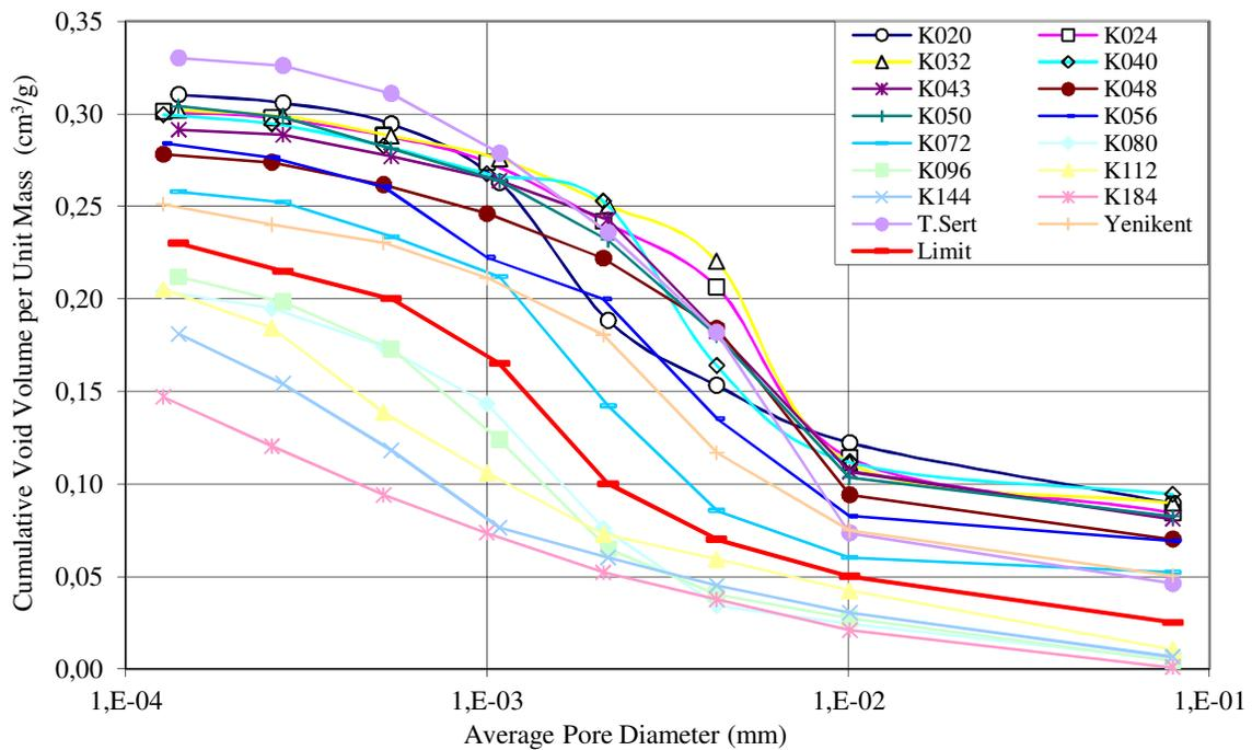
**Figure 9.** Average pore diameter variation of samples
