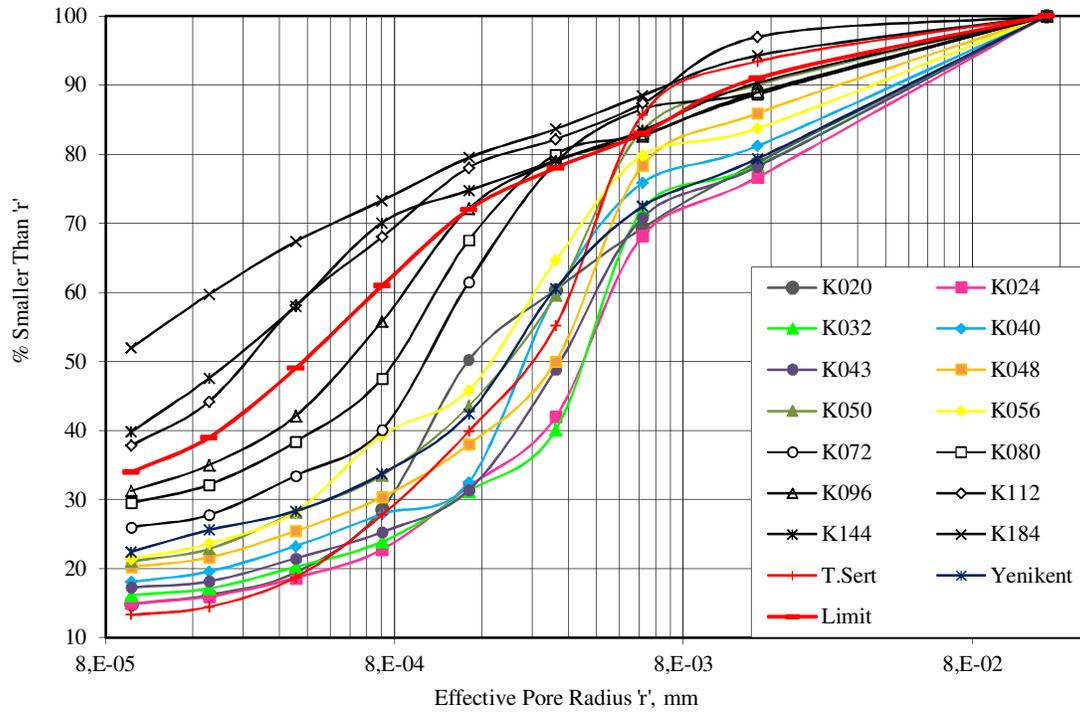
**Figure 10.** Pore size distribution curves of samples
