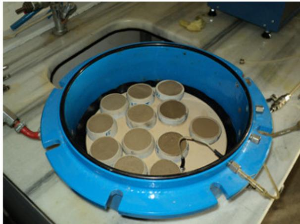
**Figure 6.** Pressure plate soil samples
