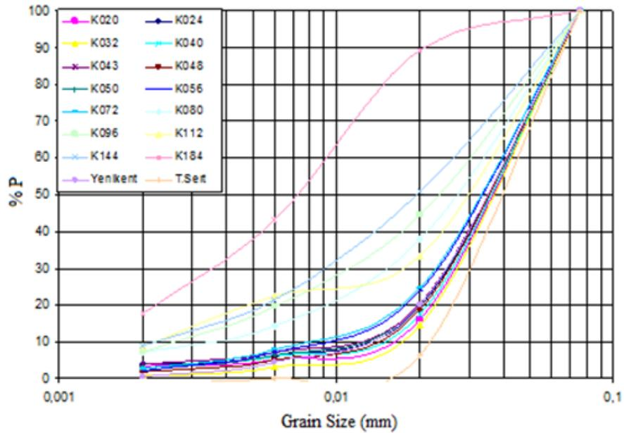
**Figure 3.** Grain size distribution of silt mixtures
