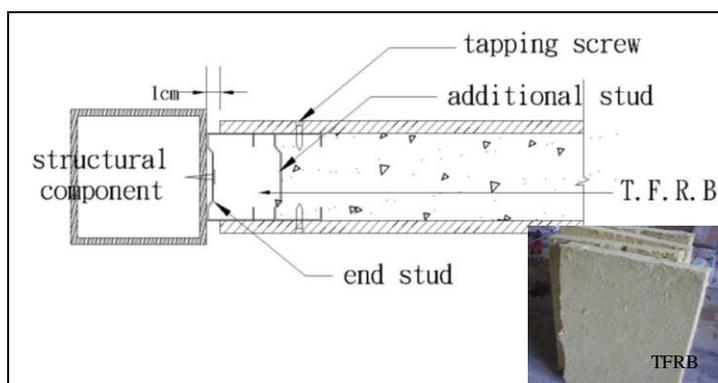
**Figure 5.** Details of the W6 specimen
