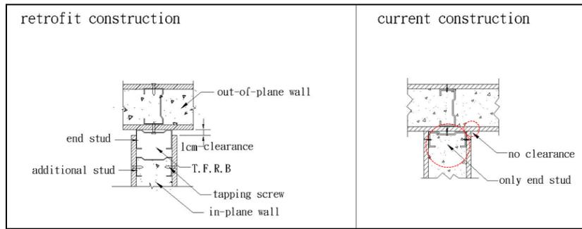
**Figure 7.** Retrofit construction in T shape wall
