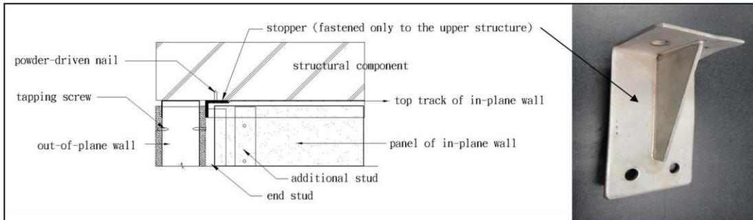
**Figure 8.** Details at the top junction of two walls in W8 specimen
