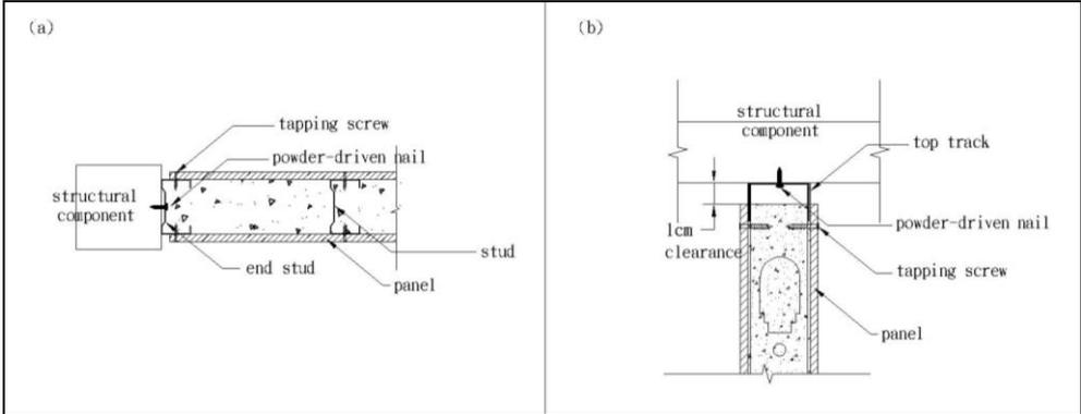
**Figure 2.** Details of the end stud (a) and the top track (b)
