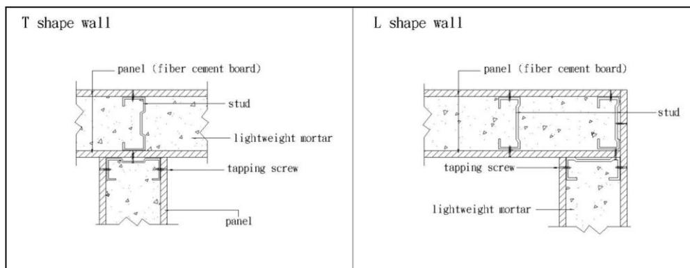
**Figure 4.** Detailed connections of the T shape wall and the L shape wall
