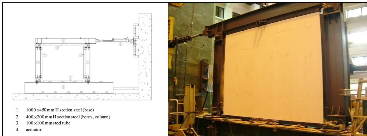
**Figure 3.** Details of the test frame
