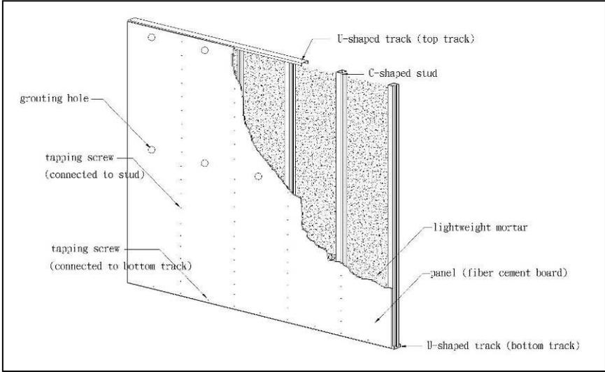
**Figure 1.** Typical construction of the DMF system
