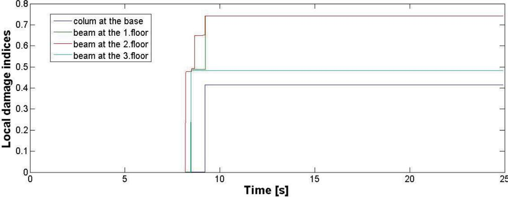
Figure 4.5. Evolution of the local damage indices of selected elements during earthquake
