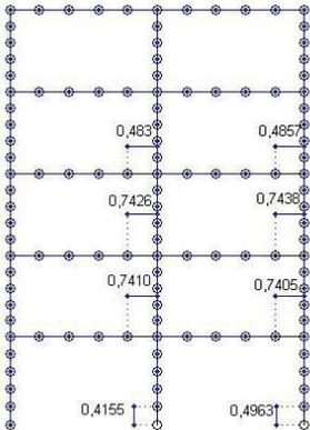
Figure 4.4. Local damage index distribution along the entire structure at the end of seismic loading
