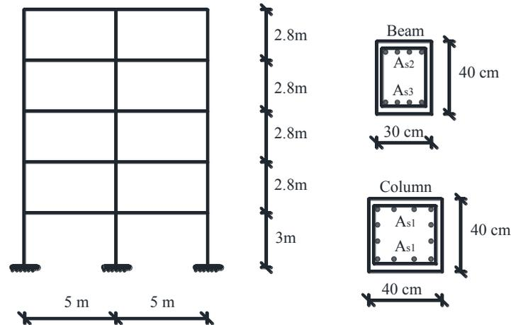
Figure 4.1. Geometry, reinforcement and cross-sections of the reinforced concrete frame
