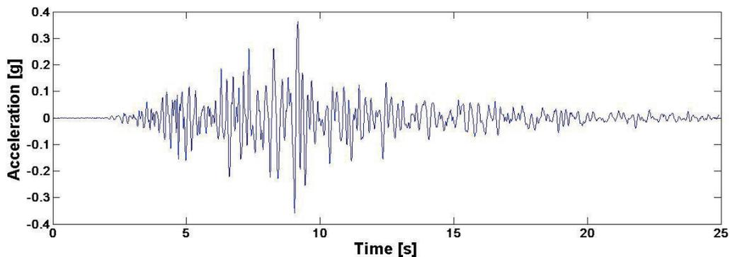
Figure 4.2. Accelerogram of the Kobe earthquake, Japan, 1995
