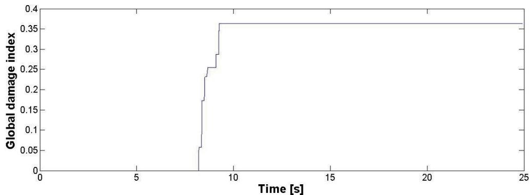
**Figure 4.6.** Evolution of the global damage index during the earthquake
