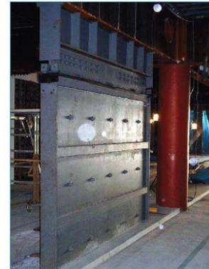
**Figure 4.** Structural framing diagram and photos of energy dissipation members
