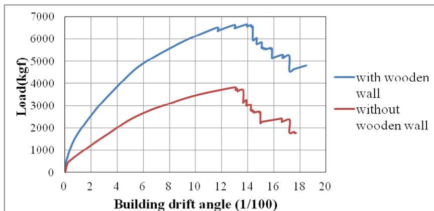
Figure 23. The contribution of the wooden panel wall
