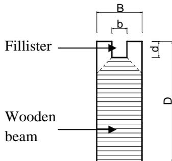
**Figure 9.** The Cross-sectional detail of the beam
