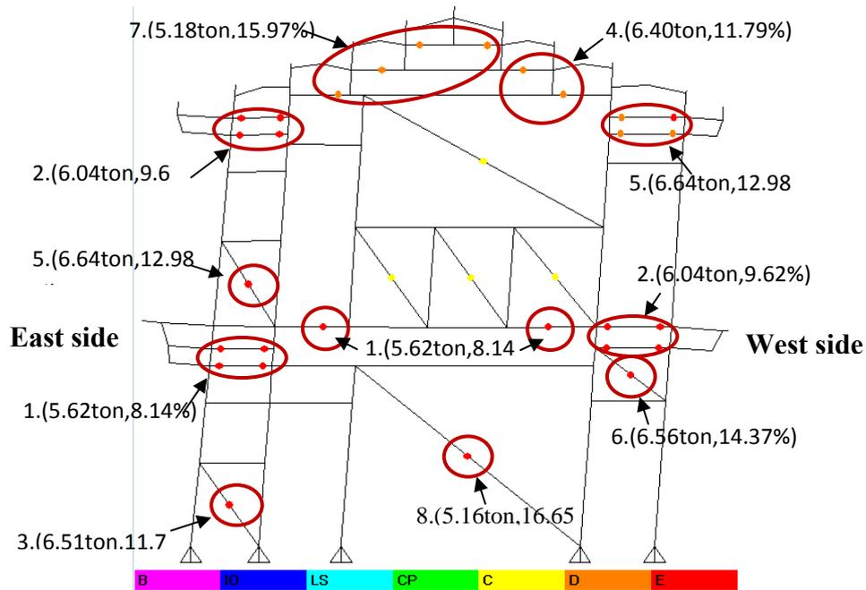
Figure 22. The damage mode of the frame when the drift angle on the roof reach 0.171
