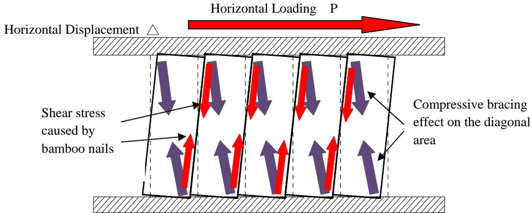
**Figure 3.** In-plane behavior of the wooden panel under horizontal load
