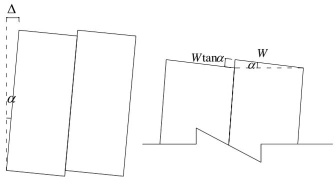
Figure 12. The shear deformation of bamboo nails
