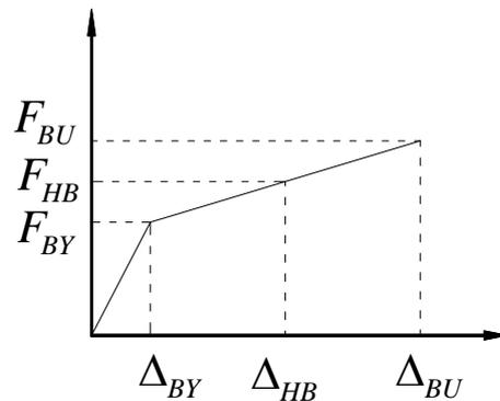
**Figure 10.** The force-deformation relationship of the unit length of the beam
