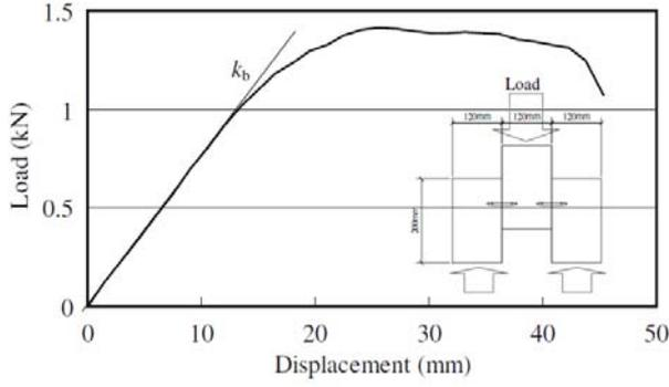
**Figure 13.** Loading–displacement relation of bamboo nail(Chang ,2007)
