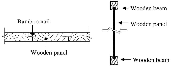
**Figure 2.** Connection details of the wooden panel wall
