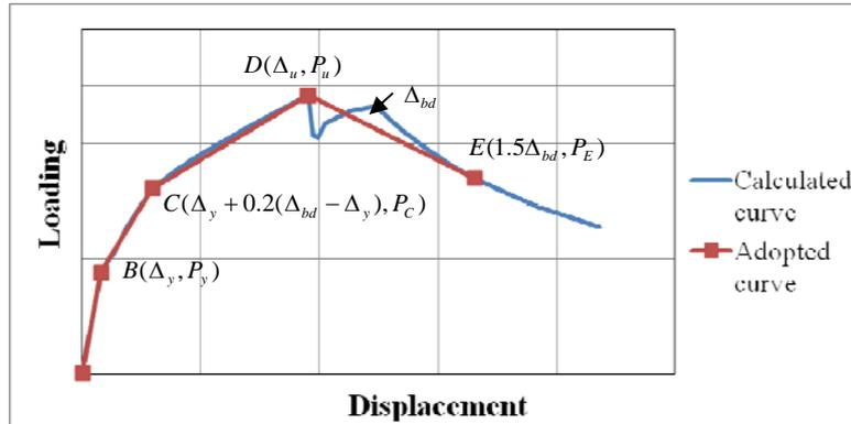
Figure 16. The adopted loading-displacement relationship curve of the modeling compressive brace
