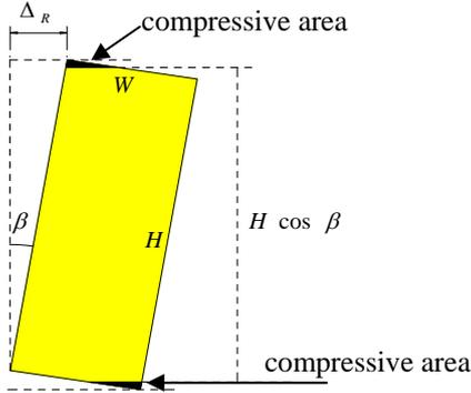
**Figure 7.** The displacement caused by the compressive deformation of the beam
