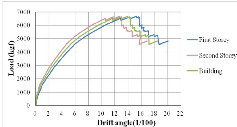
**Figure 24.** The comparison of the drift angle of different storey
