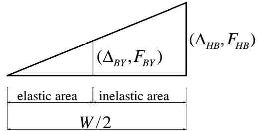
**Figure 8.** The deformation assumption of the beam
