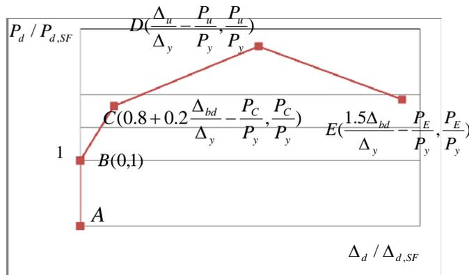
Figure 17. The plastic hinge properties setting of the modeling compressive brace
