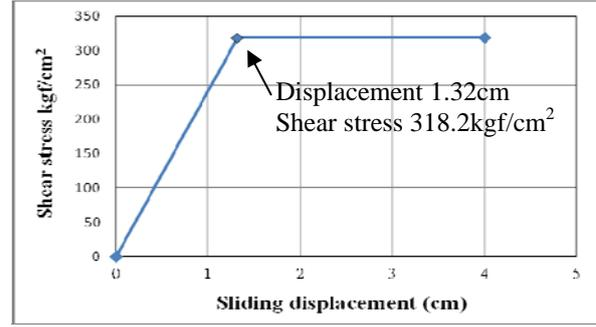
**Figure 14.** The stress-displacement relationship of bamboo nail adopted for analysis
