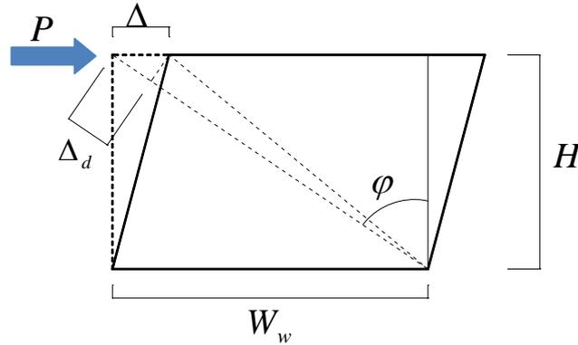
**Figure 15.** The force and deformation relationship between wall and compressive brace
