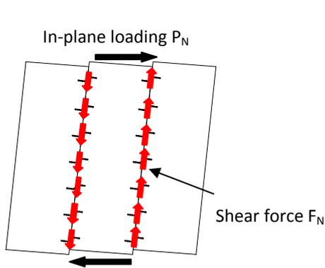
Figure 11. The shear force of bamboo nails
