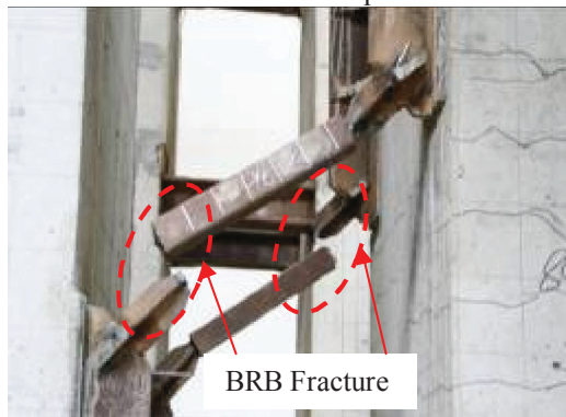
Figure 4.5. B2 fracture at specimen TRC-BRB at 240mm displacement
