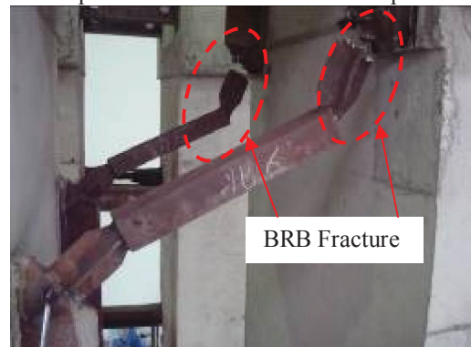
Figure 4.6. B6 fracture at specimen TRC-BRB at 110mm displacement
