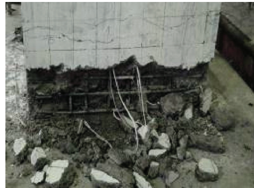
Figure 4.2. Concrete cover spalling at the west side of specimen SRC at 190mm displacement
