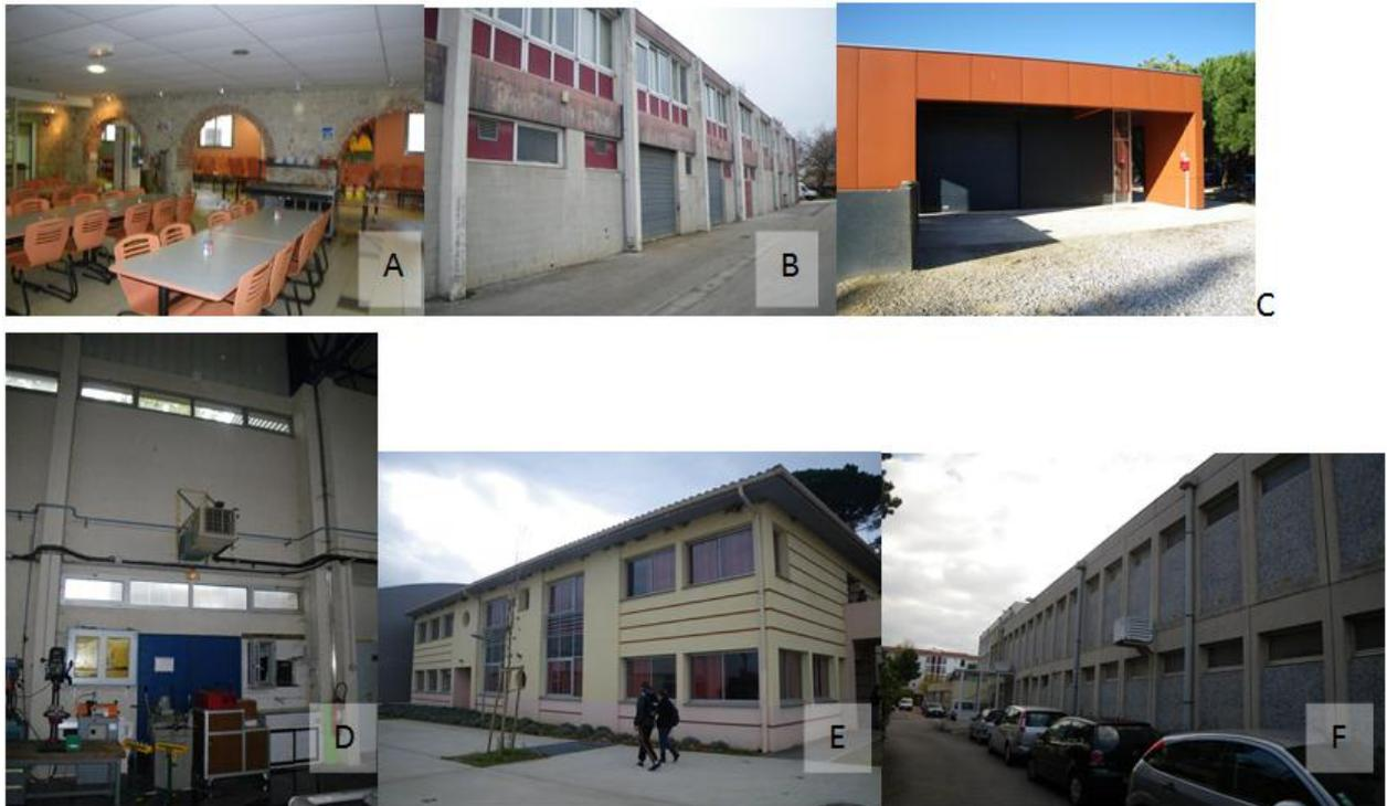
**Figure 2.2.:** parameter WA, examples of different structural systems. A) Traditional stone and brick U masonry, B) RC frames and infill walls, C) wood structure, D) steel structure and infill walls, E) masonry and RC structure and F) prefabricated building.
