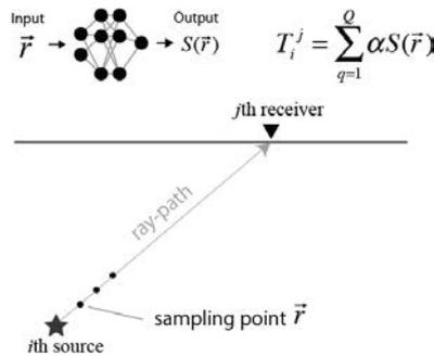
**Figure 1.** Schematic diagram of the travel time computation. First, the slowness at all sampling points along a ray path is obtained by the neural network, and the travel time is then calculated using Eqn. 2.2.
