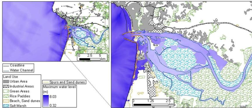
**Figure 4.4.** Maximum water level at Figueira da Foz, obtained by removing the spurs and sandy dunes.
