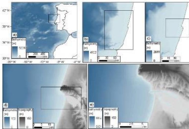
**Figure 2.2.** Nesting used to calculate the tsunami inundation at Figueira da Foz: a) cell size of 2025 m; b) cell size of 675 m; c) cell size of 225 m; d) cell size of 75 m; e) cell size of 25 m.
