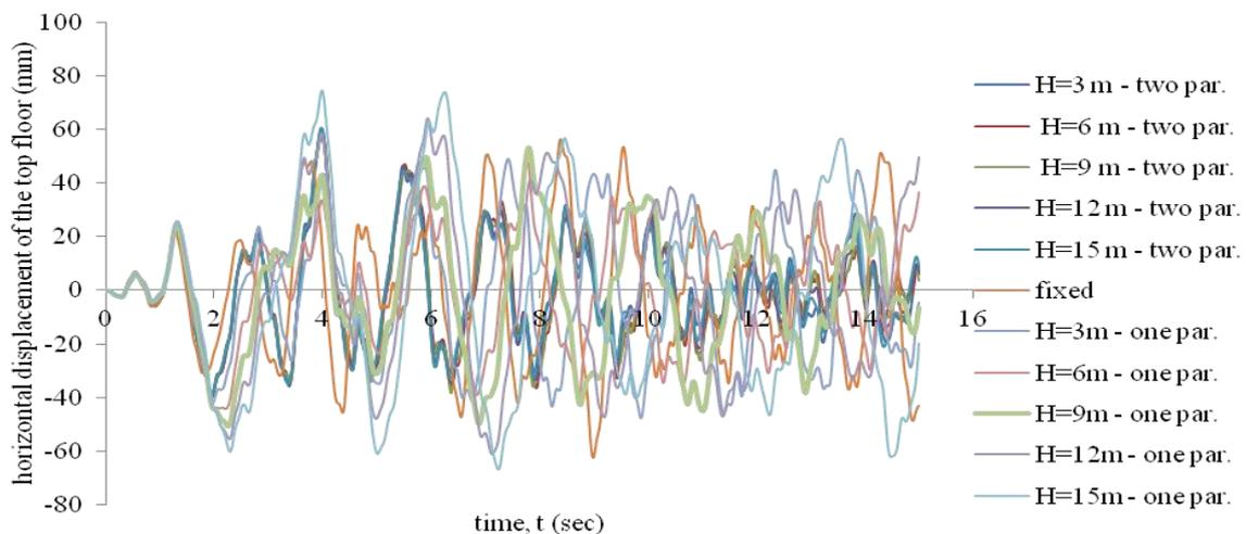
**Figure 3.3.** Variation of top floor horizontal displacement in earthquake direction with time and compressible subsoil depth (H)
