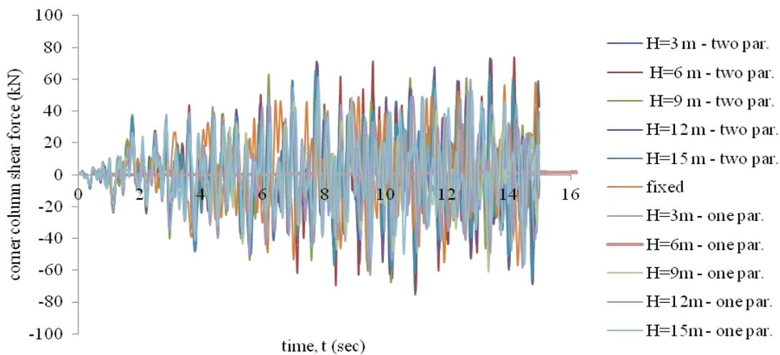
**Figure 3.4.** Variation of corner column base shear with time and compressible subsoil depth (H)
