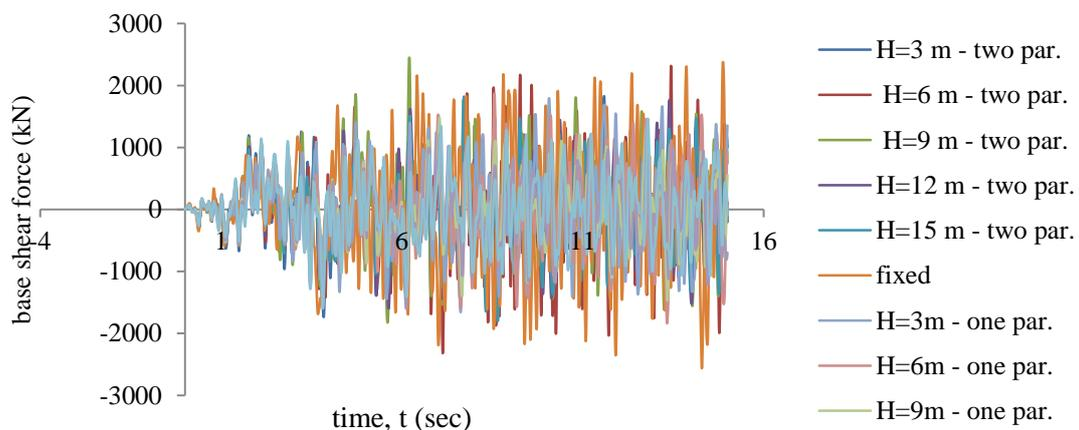
**Figure 3.6.** Variation of total base shear with time and compressible subsoil depth (H)
