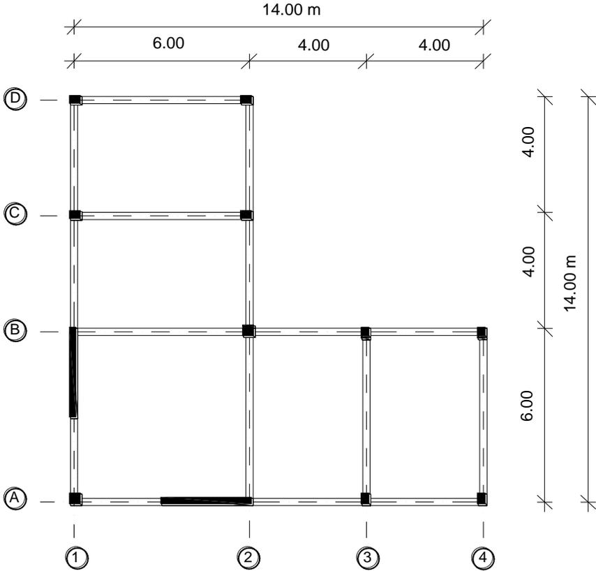
Figure 3.1. Plan view of the 3D building
