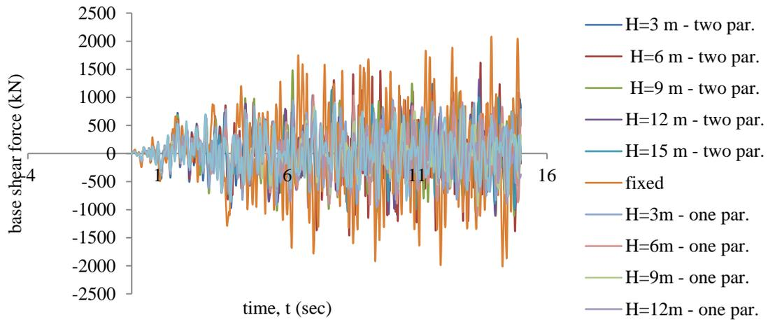
**Figure 3.5.** Variation of base shear of shear-wall with time and compressible subsoil depth (H)
