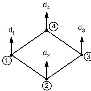
**Figure 2.1.** Four d.o.f. subsoil shear element
