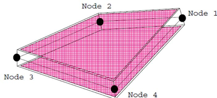
**Figure 3.2.** Shell4N element used to model the masonry structures in this study, SLang (2004)
