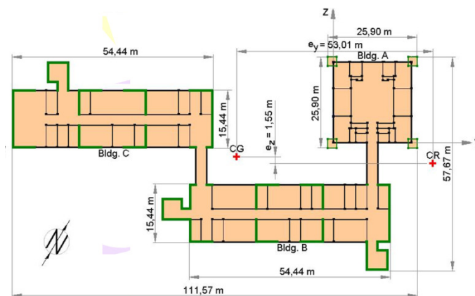
Figure 4.8. Eccentricity between two intrinsic centres after structural interventions-hypothesis without seismic joints
