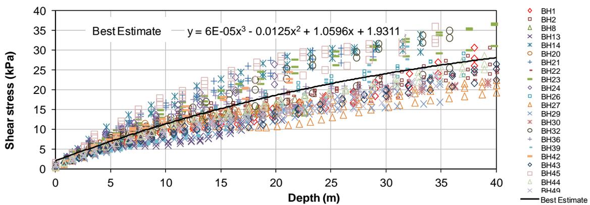
**Figure 3.** Maximum shear stress against depth for all boreholes for ‘10% chance of being exceeded in the next 50 years’ ground motion
