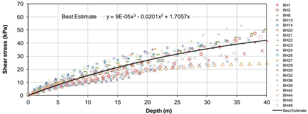
**Figure 5.** Maximum shear stress against depth for all boreholes for ‘2% chance of being exceeded in the next 50 years’ far-field ground motion
