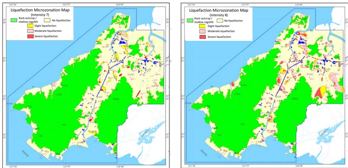
**Figure 8.** Contours of liquefaction probability based on the Chinese Seismic Code (GB50011-2010) for (a) earthquake Intensity 7 and (b) Intensity 8 ground motions
