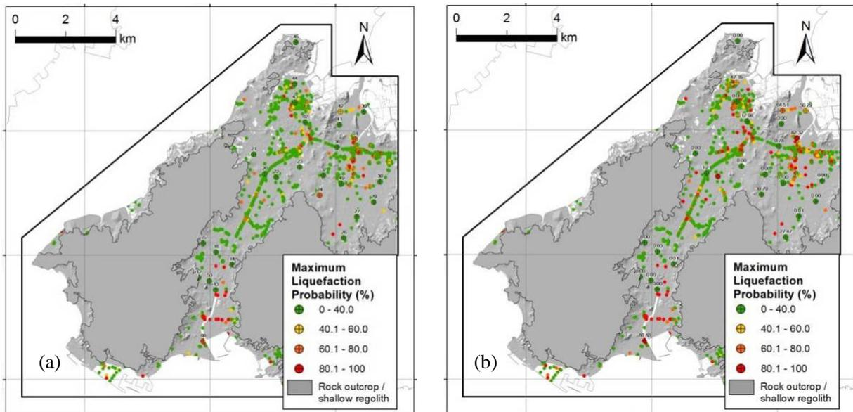
Note: Area with rock outcrop / shallow regolith is not considered in the liquefaction assessment
