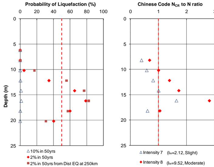
**Figure 2.** Liquefaction chart for borehole no. BH01
