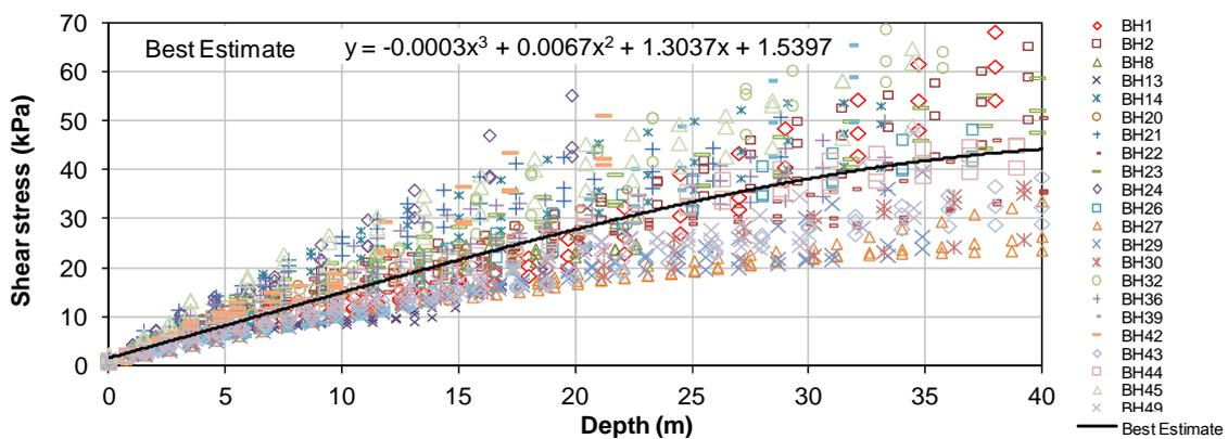
**Figure 4.** Maximum shear stress against depth for all boreholes for ‘2% chance of being exceeded in the next 50 years’ near-field ground motion
