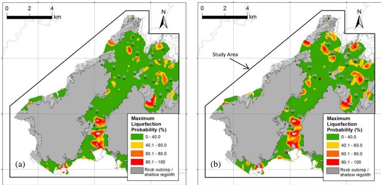
**Figure 7.** Contours of liquefaction probability based on best estimate design lines for ‘2% chance of being exceeded in the next 50 years’ (a) near-field and (b) far-field earthquake ground motions
