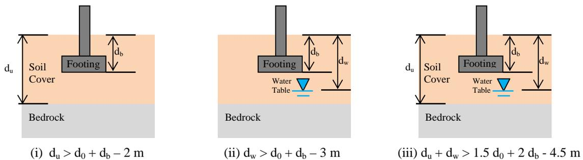
**Figure 1.** Illustration of the non-liquefaction criteria for covering soil and level of ground water
