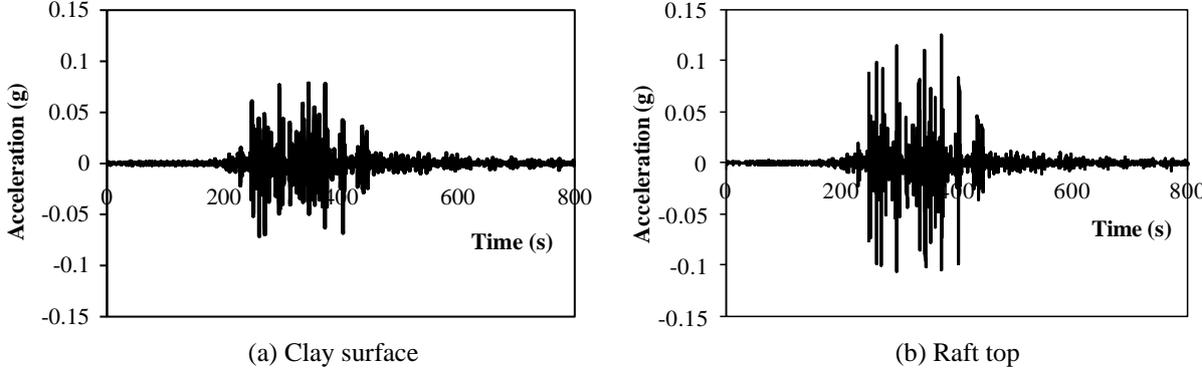
**Figure 8.** Measured accelerations at clay surface and raft top for 2 × 1 compact pile group
