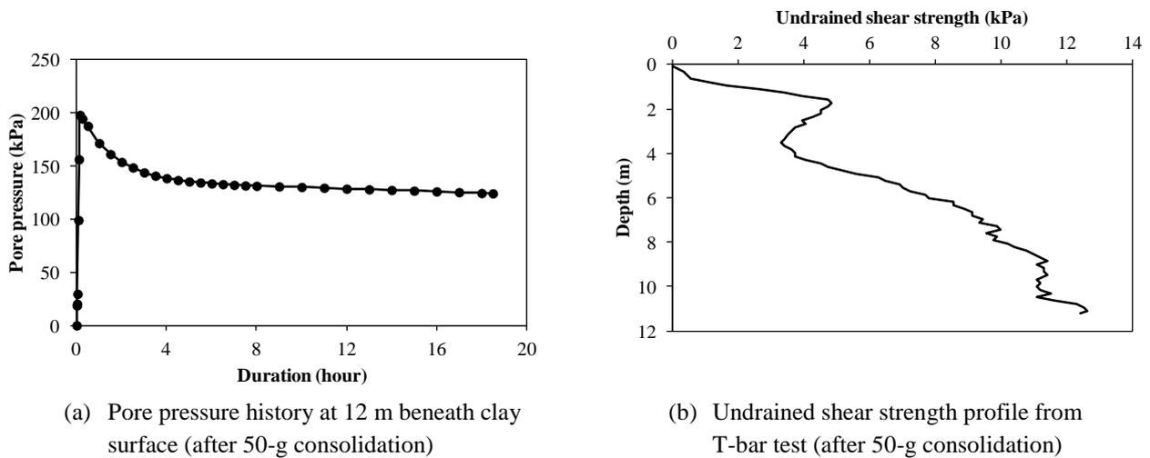
**Figure 6.** Pore Pressure History and Shear Strength Profile after 50-g Consolidation Phase
