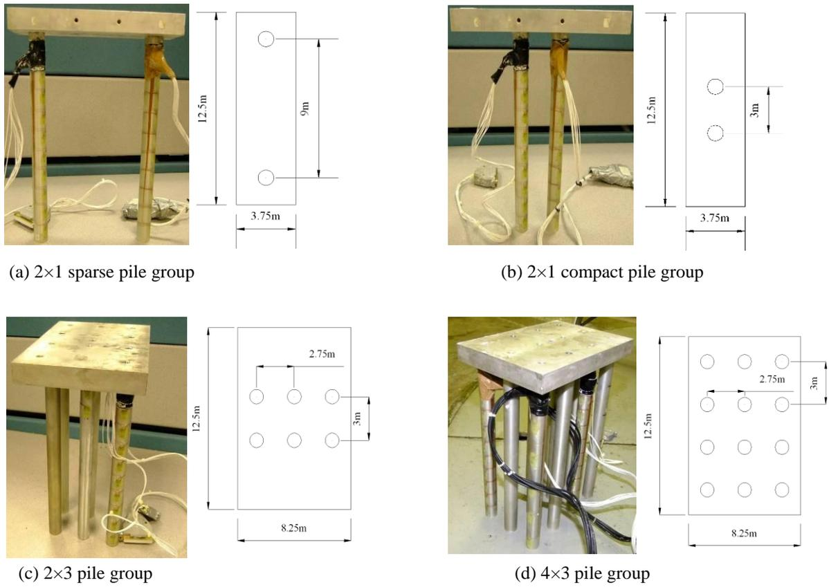
**Figure 4.** Photo and schematic plan view of pile-raft system (prototype dimensions)
