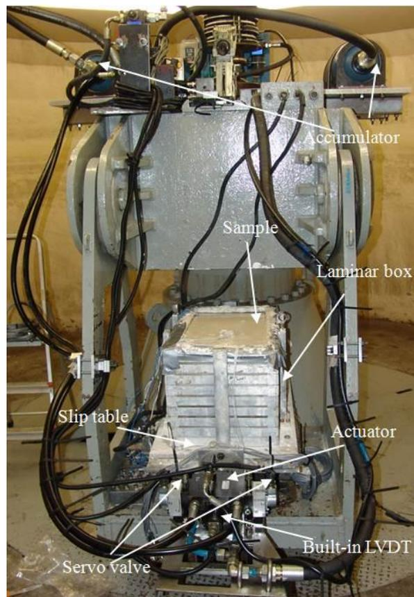
**Figure 3.** Centrifuge shaking table with test model on swing platform
