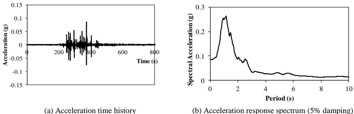
**Figure 7.** Typical measured acceleration time history at the model base and its response spectrum
