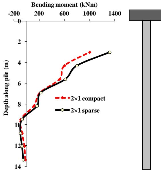
**Figure 10.** Measured maximum bending moment profiles for 2×1 sparse and 2×1 compact pile groups
