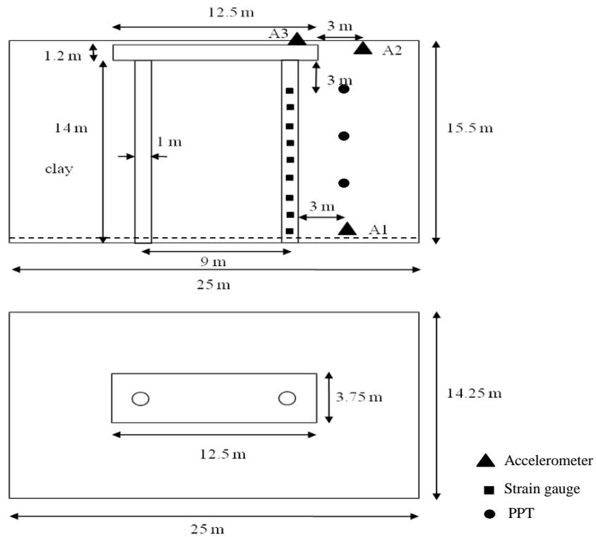
**Figure 5.** Schematic layout for the sample of 2×1 sparse pile group (prototype dimensions)
