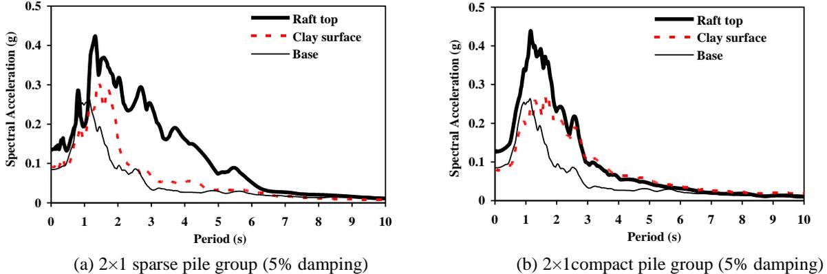
**Figure 9.** Acceleration response spectra at different locations for 2x1 sparse and compact pile groups
