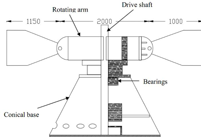
**Figure 2.** Schematic view of NUS geotechnical centrifuge (after Banerjee, 2009)
