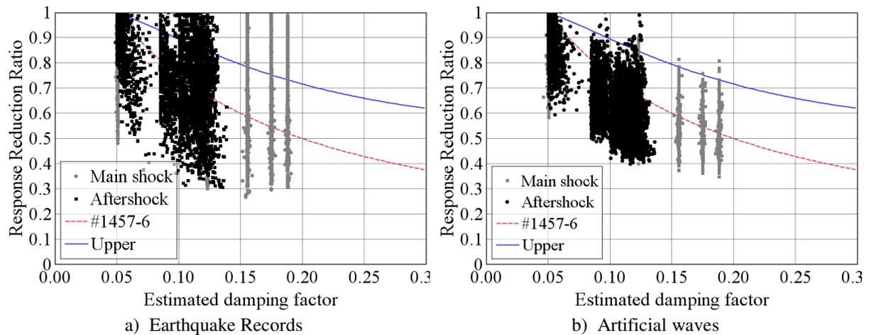
**Figure 4.3.** Relationship between response reduction ratio and estimated damping factor for Takeda Model
