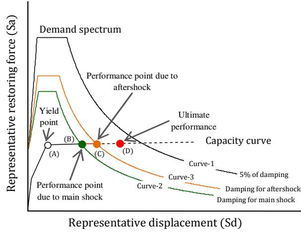
**Figure 1.1.** Capacity curve and Demand curve
