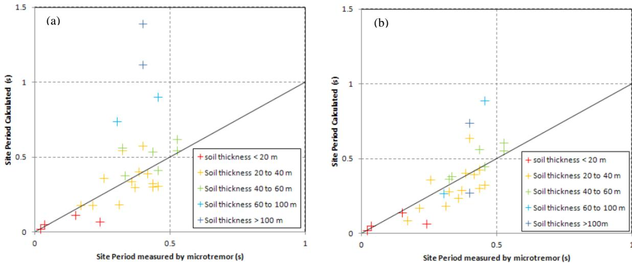
**Figure 4.** Comparison between measured and calculated site periods when considering (a) the entire profile, (b) down to where the SPT N value is > 100
