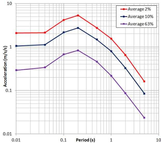
**Figure 7.** Average bedrock UHRS target spectra
