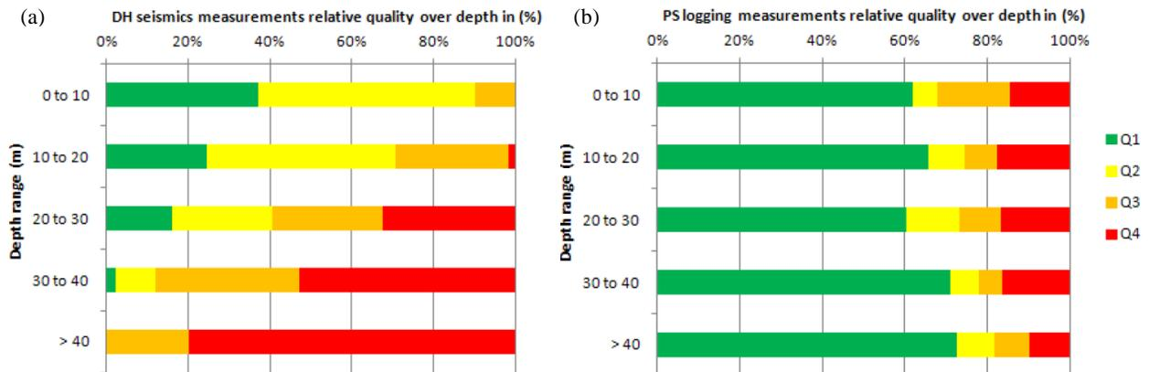
Figure 3. Downhole seismic vs. PS logging measurements relative quality with depth
