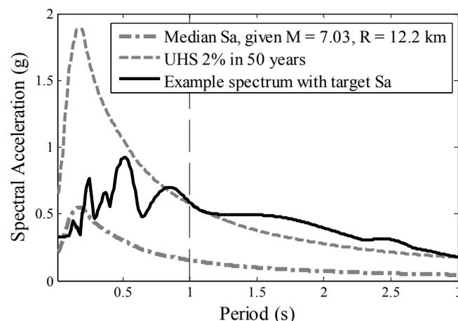
**Figure 1.** Median predicted spectrum having  $M=7.03$  and  $R=12.2$  km. UHS for 2 % probability of exceedance in 50 years. The example spectrum is the Newhall-W Pico Canyon Rd with  $M=6.7$  recorded from Northridge event (PEER 2010).
