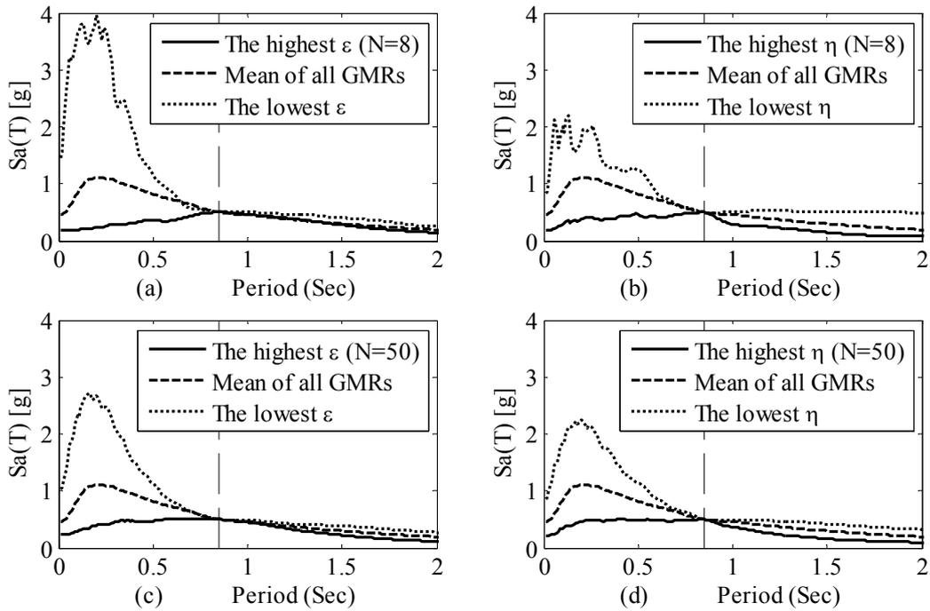
**Figure 2.** Comparison of the mean spectrum based on 534 GMRs with (a) the mean spectrum based on *N*=8 highest/lowest Epsilon, (b) the mean spectrum based on *N*=8 highest/lowest *Eta*(PEER), (c) the mean spectrum based on *N*=50 highest/lowest Epsilon, (d) the mean spectrum based on *N*=50 highest/lowest *Eta*.
