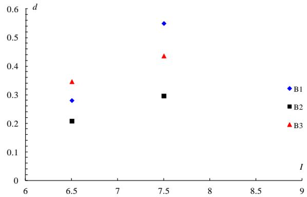
**Figure 3.1.b.** Average normalized damage grade versus macroseismic intensity
