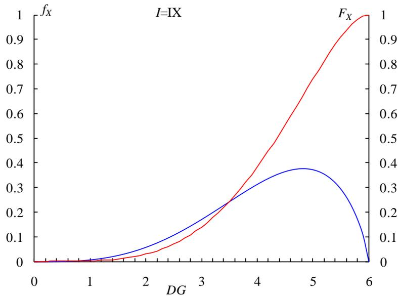
**Figure 4.1.** B1 building typology - probability functions of damage grades for seismic intensity IX
