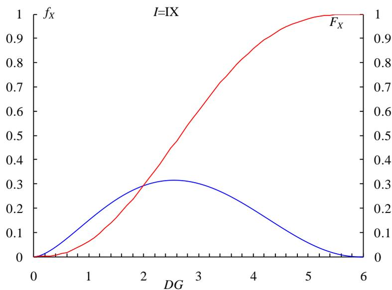
**Figure 4.2.** B2 building typology - probability functions of damage grades for seismic intensity IX
