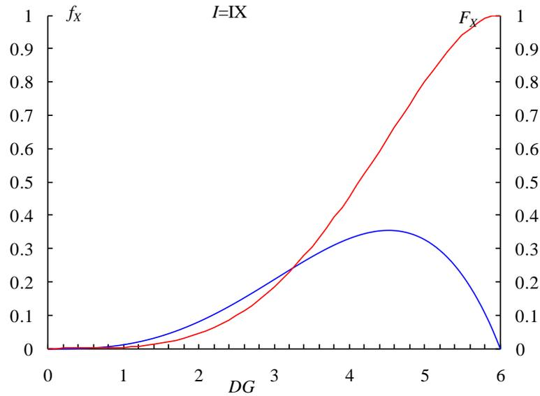
**Figure 4.3.** B3 building typology - probability functions of damage grades for seismic intensity IX
