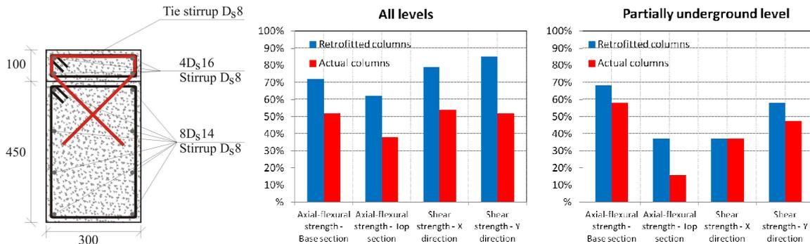
**Figure 10.** Inadequacy of r.c. structure in terms of safety ratio (i.e. percentage of column that verifies safety without dissipative elements). Red actual configuration, blue upper floors strengthening and mass reduction.
