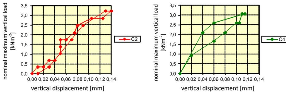
**Figure 6.** Vertical load-displacement results for second floor (left) and fourth floor (right) static load tests
