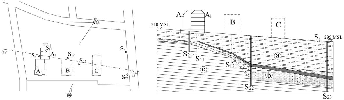
**Figure 1.** Geological survey's results at design time (1984): housing area and drilling positions (first series  $S_{1i}$ , second series  $S_{2i}$ ), geological section (W-E) with stratigraphical profile and natural ground slope ( $\approx 12.5\%$ )
