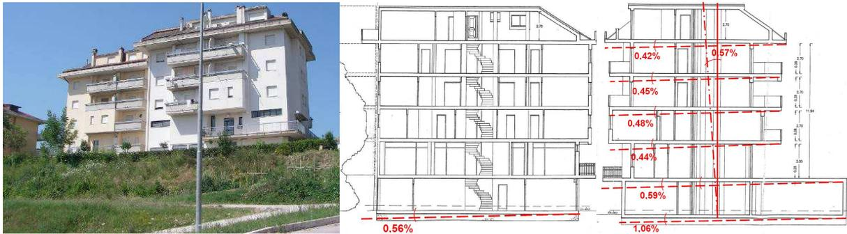
**Figure 2.** View of the study building (right side building) with the twin one (left side); longitudinal (S-N) and transverse (W-E, like geological one) sections of building with vertical sloping
