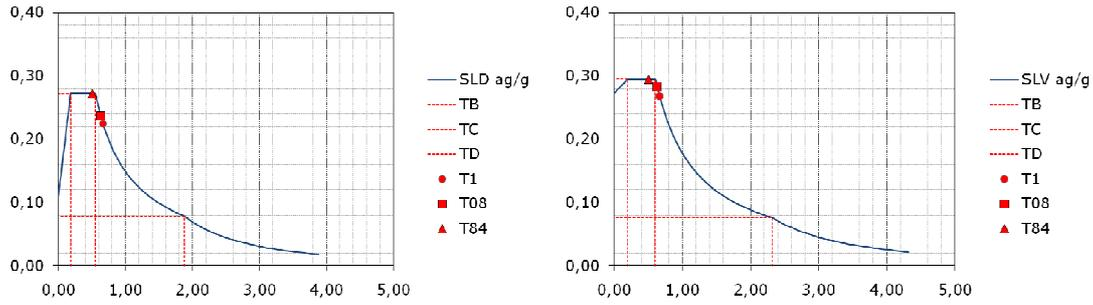
**Figure 8.** Design spectra for study building at SLD (elastic, left) and at SLV ( $q = 2.25$ , right)
