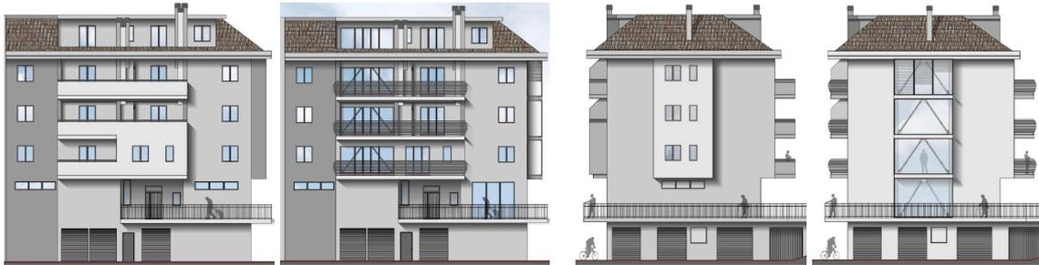
**Figure 9.** Mass removing hypotheses for East (left) and North building fronts (right) of the study building
