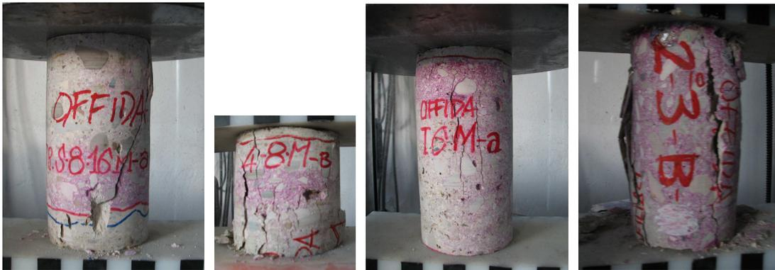
**Figure 4.** Concrete drilled cores after compressive tests: lower strength cores (S 8-16 M-a & 4-8 M-b [left]), medium strength core (T6 M-a [centre]) and highest strength core (2-3 B [right])
