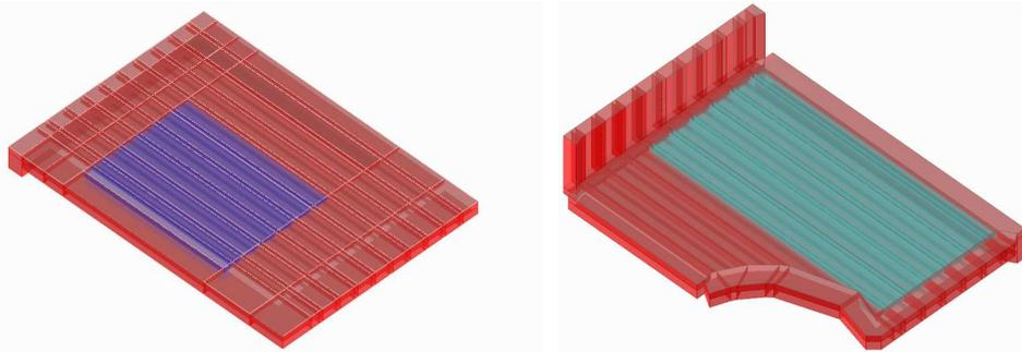
**Figure 7.** Linear Fem models for second (left) and fourth (right) tile-lintel horizontal floors
