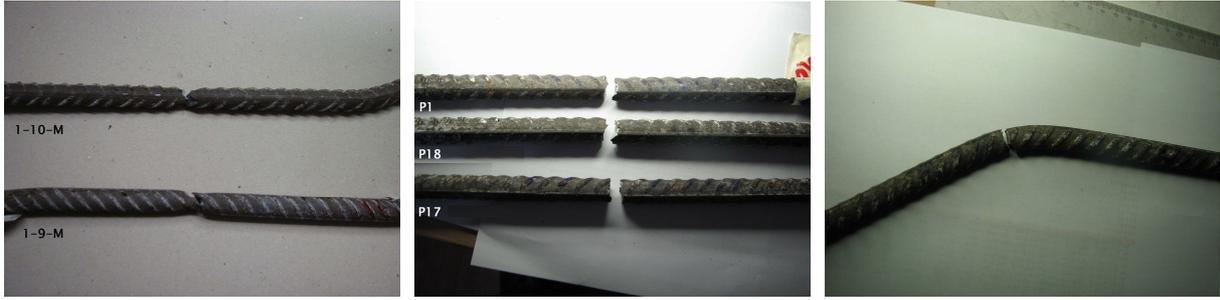
**Figure 3.** Steel reinforcement ( $D_s = 14 \text{ mm}$  left) after tensile tests and bend test: low ductility is detected in  $D_s = 16 \text{ mm}$  rebars (centre and right). Good ductility in  $D_s = 14 \text{ mm}$  rebars
