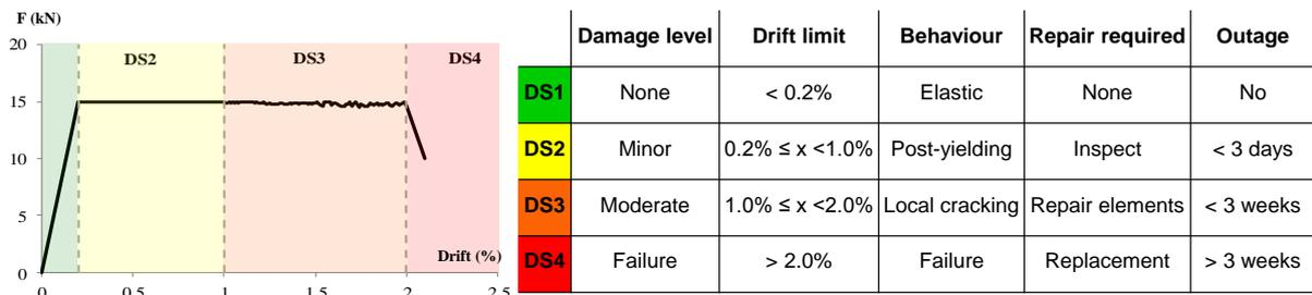
**Figure 3.4.** Damage states definition
