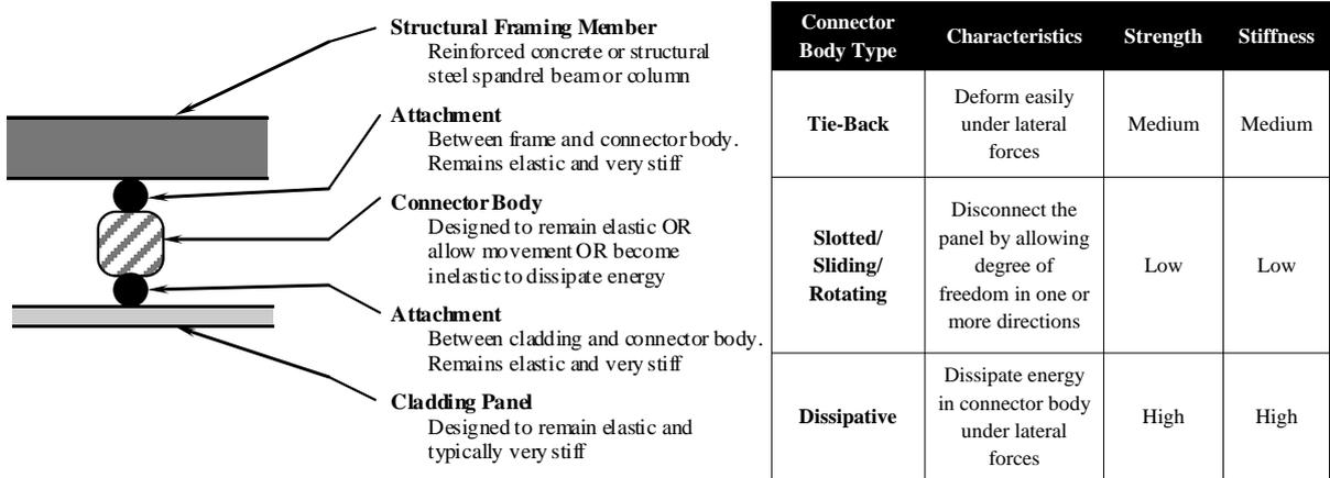
Figure 2.2. Cladding system composition (left) (Pinelli et al., 1993), typical connector body types (right)
