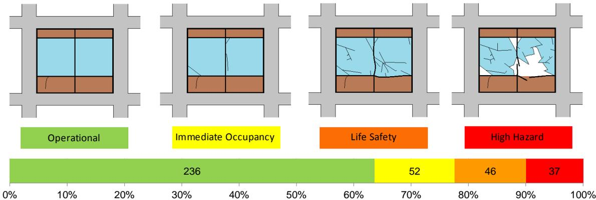
**Figure 2.1.** Graphical representation of cladding performance levels (top) and facade performance composition following Christchurch 22/02/2011 earthquake
