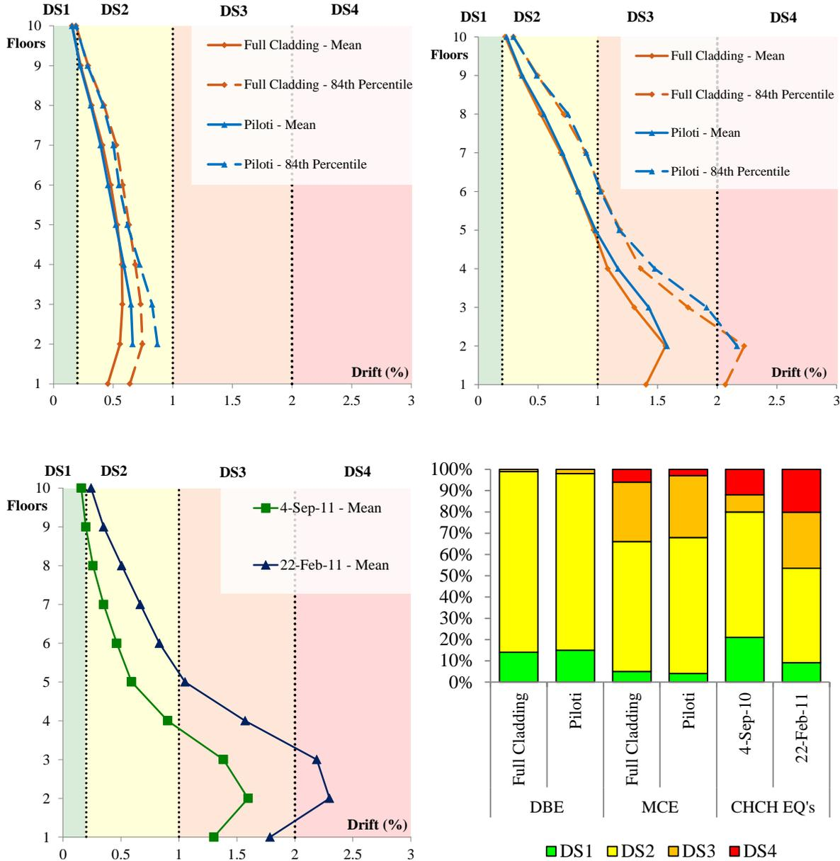
**Figure 5.5.** Differential displacement between panel and frame and corresponding connection damage state for DBE (top left), MCE (top right) and Christchurch Earthquakes (bottom left) and damage state composition (bottom right)
