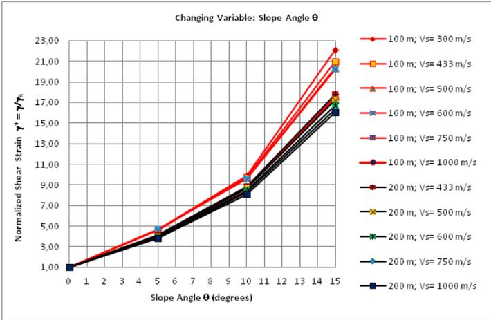
Figure 4.5. Sensitivity analysis based on slope angle with AMPLE2
