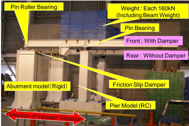
**Figure 3.1.** Set up of the tests
