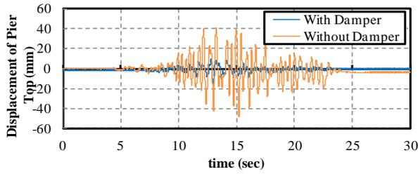
**Figure 4.4.** Waveform for displacement of the top of the bridge pier Bridge pier (T-I)
