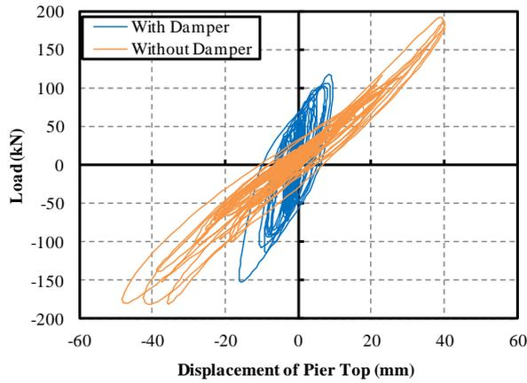
**Figure 4.6.** Load - displacement relationship (T-I)
