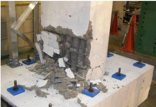
**Figure 4.11.** Damage to bridge pier base by T-II motion without dampers
