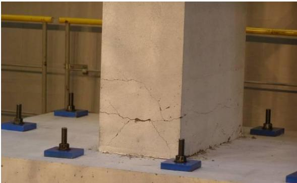
**Figure 4.10.** Damage to bridge pier base by T-I motion without dampers
