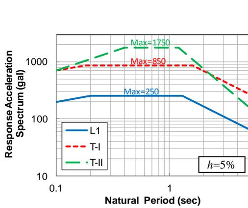
Figure 3.5. Response spectra of input motions
