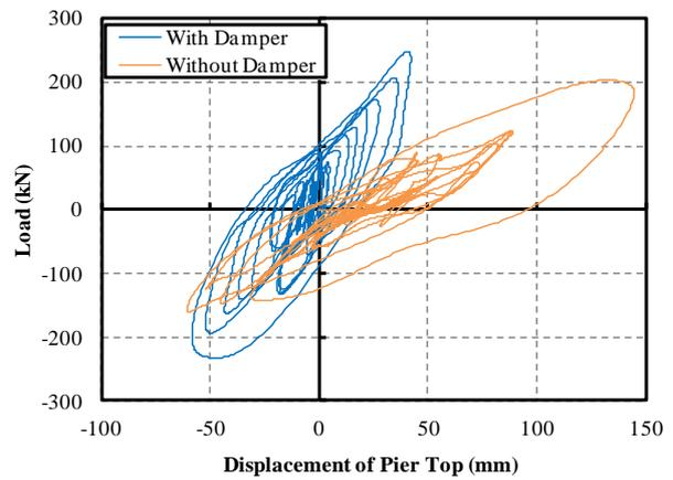
**Figure 4.7.** Load - displacement relationship
