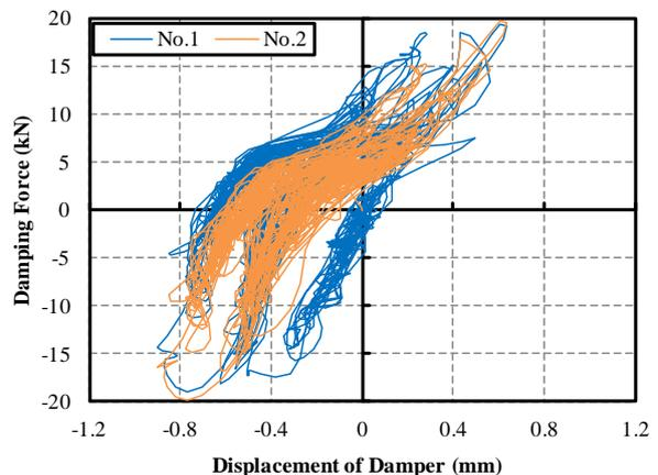
Figure 4.3. Damping force - displacement relationship of dampers (L1)
