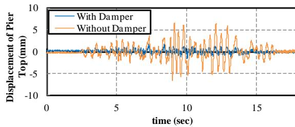
Figure 4.1. Waveform for displacement of the top of the bridge pier Bridge pier (L1)
