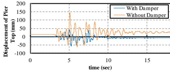
**Figure 4.5.** Waveform for displacement of the top of the bridge pier Bridge pier (T-II)
