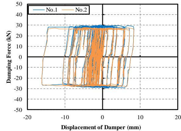
**Figure 4.8.** Damping force - displacement relationship of dampers (T-I)
