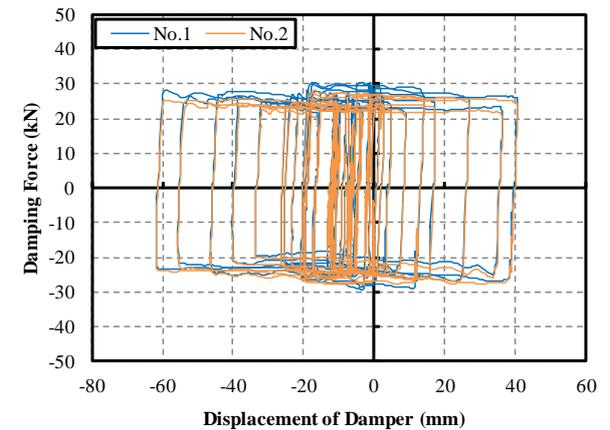
**Figure 4.9.** Damping force - displacement relationship of dampers (T-II)
