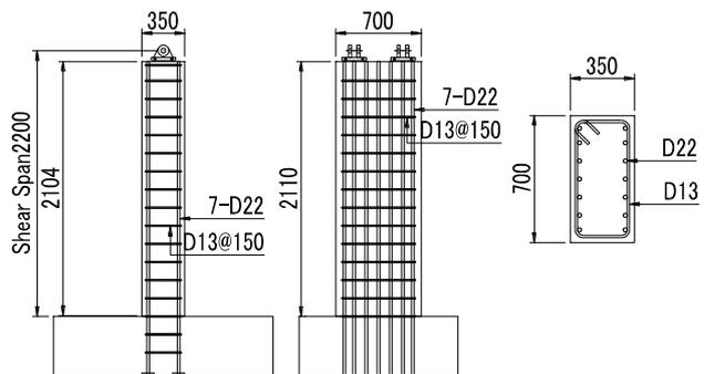
**Figure 3.4.** Bridge pier model
