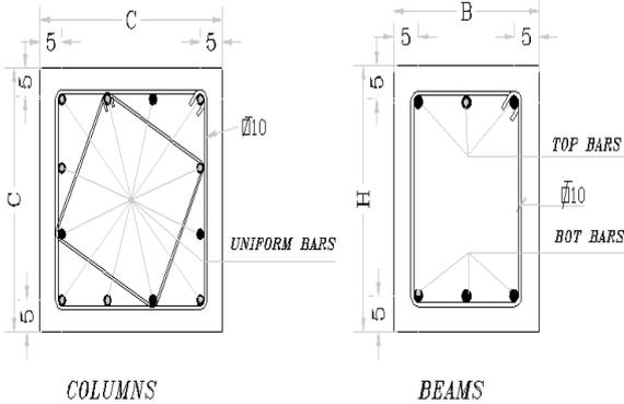
**Figure 3.1.** Cross sections of beams and columns
